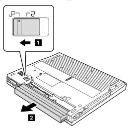
When installing: Install the battery pack along the slide rails on the left and right sides of the battery-pack slot. Then make sure that the battery latch is locked.
