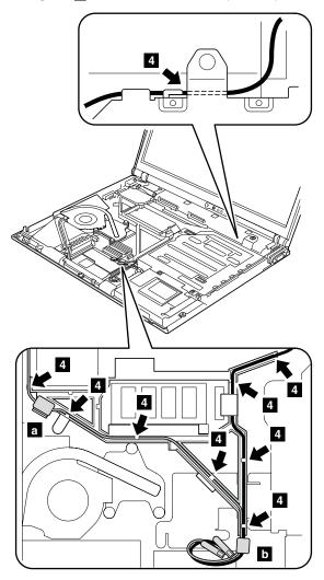
When installing: Make sure that the antenna cables and the two ferrite cores **a** and **b** (with sponge) are correctly routed and securely in place.
