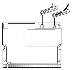
Insert the notched end of the card into the socket, and then press the card firmly. Pivot the card until it snaps into place. Make sure that it is firmly fixed in the slot and does not move easily.
