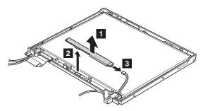
When installing: Make sure that connectors 2 and 3 are firmly attached.
