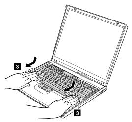
Make sure that all the projections on the front side of the keyboard b are firmly attached under the frame.
