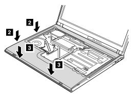
3. Secure the keyboard bezel from the underside of the computer with the screws.
