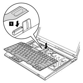
2. Install the keyboard so that the keyboard edges are under the frame.
