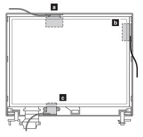
2. Route the antenna cables as in the following drawings:
