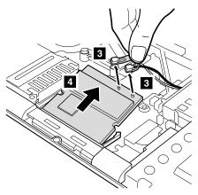
When installing: Plug in the wireless antenna cable as follows:
