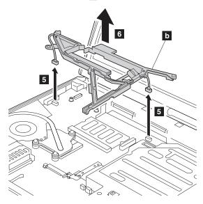
When installing: Make sure that the connectors **5** are firmly attached.
