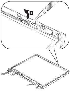
Lift the latch bar in the direction of the arrow 2, and then remove the left latch in the direction of the arrow 3.
