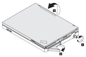
Release the latches to remove the battery pack.
