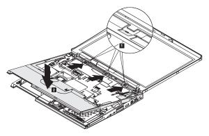
Note: After installing upper case, please arrange antenna as shown below.
