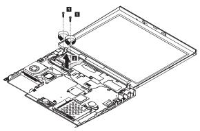
Then remove the two screws at the rear side.
