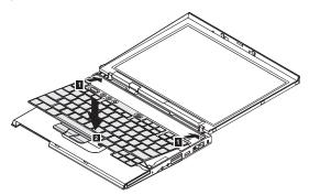
To make sure that the front side of the keyboard is housed firmly, gently press the keys with your thumbs and try to slide the keyboard toward you.
