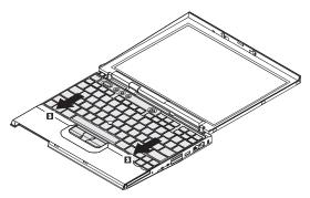
4. Secure the keyboard by tightening the screws from the bottom side of the computer.
