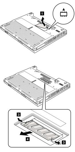
When installing: Insert the notched end of the DIMM into the socket. Press the DIMM firmly, and pivot it until it snaps into the place.
