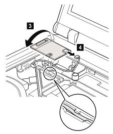
When installing: Make sure that connector 4 and the connector on the underside of the card are firmly attached. Then place the cable to fit in the cable guide as in the figure.
