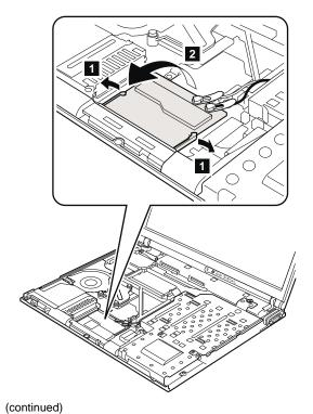
**Note:** When unplugging the antenna jack, do not pull the cable; it might snap. Unplug the jack by pulling the tab with your fingers.
