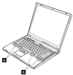
Secure the keyboard from the underside of the computer, using the new screws provided with the keyboard.
