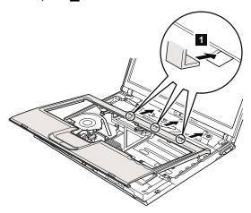
While inserting the three latches, align the top-left corner of the keyboard bezel as in figure  ${f a}$ .
