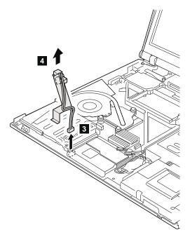
Remove the connector 3 . And strip the tape securing the IEEE 1394 cable to the PC Card slot and remove the IEEE 1394 cable 4.
