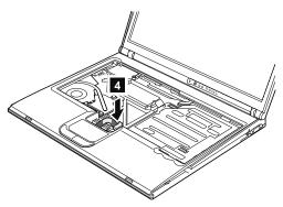
Secure the keyboard bezel from the underside of the computer with the screws.
