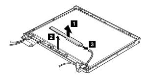
When installing: Make sure that connectors 2 and 3 are firmly attached.
