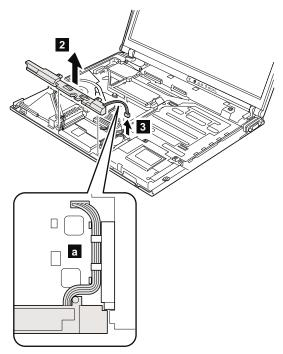
When installing: Make sure that the connector 3 is firmly attached. Then route the cable as in a .
