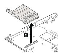
When installing: Make sure that the connector 2 is firmly attached to the system board.
