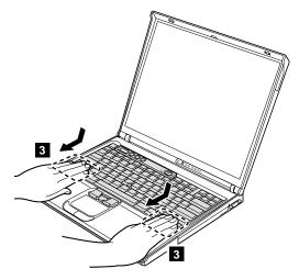
Make sure that all the projections on the front side of the keyboard are firmly attached under the frame.
