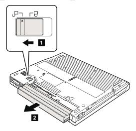
When installing: Install the battery pack along the slide rails on the left and right sides of the battery-pack slot. Then make sure that the battery latch is locked.
