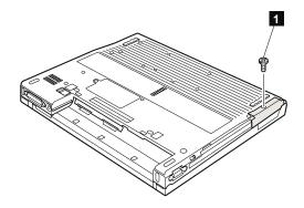
Note: The hard disk is attached to the cover.
