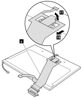
Removing and replacing a FRU Remove the right latch from the LCD cover.
