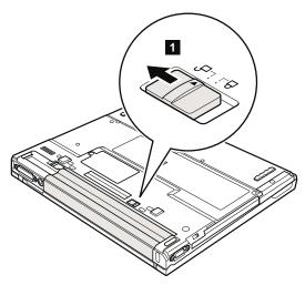
Holding the battery release lever in the unlocked position 2, remove the battery pack 3.
