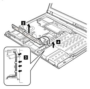
When installing: Make sure that the connector 4 is firmly attached. Then route the cable as in 3.
