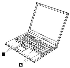
Secure the keyboard from the underside of the computer, using the new screws provided with the keyboard.
