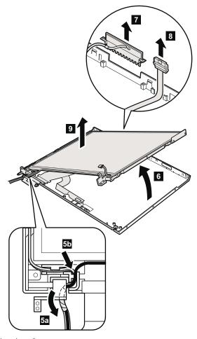
Remove the antenna assembly ( a ).
