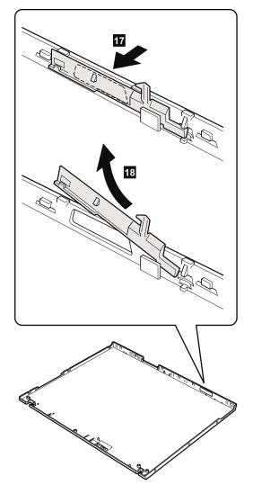
When installing: Attach the right latch to the LCD cover as follows:
