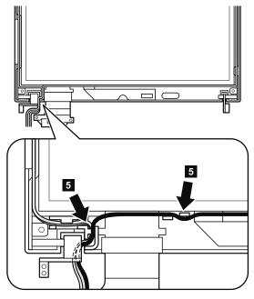
Coil the spiral tube round the antenna cables.
