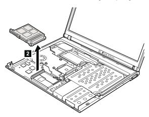
When installing: Make sure that the connector on the underside of the PC card slot 2 is firmly attached, and then secure the slot with the screws.
