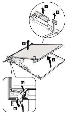
Remove the antenna assembly ( a ).
