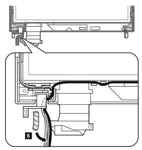
Slide the spiral tube in the direction shown by arrow  $\center{7}$ .
