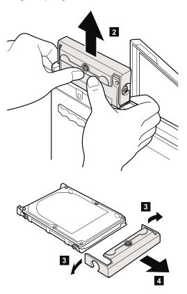
When installing: Make sure that the hard-disk connector is attached firmly.
