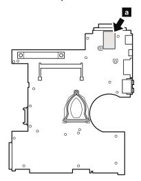
· System board without IBM security chip (bottom view)
