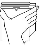
Insert the VST Zip Drive in the UltraslimBay until it is connected firmly.
