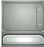
Touch Pad is feel sensitive device. It can perform all the functions of a normal mouse. Touch and move your finger on the pad to direct the on-screen pointer. The two buttons below the touch pad performs the same functions as a mouse’s two buttons.
