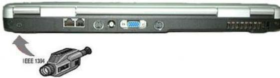
IEEE 1394 is a new data transmission standard supported by Windows systems. It can transmit data and digital videos stably and rapidly. Through the IEEE 1394 port, the computer can connect external hard disks, digital cameras and video cameras.
