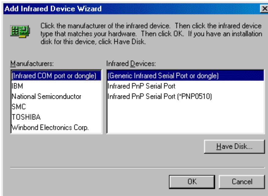
Figure 2. Select the IR device's manufacturer.
