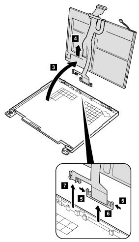
**Cable routing:** When installing the LCD, route the connector cable as in the following figure:
