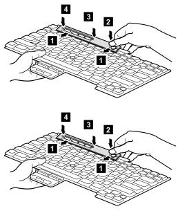
When installing the keyboard, do as follows:
