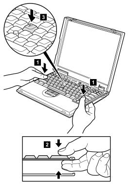
To make sure that the front side of the keyboard is housed firmly, gently press the shift keys with your thumbs and try to slide the keyboard towards you. Do not push parts (A) and (B) on the keyboard strongly; to do so might cause distortion of the Ultrabay 2000 slot and the PC Card slot.
