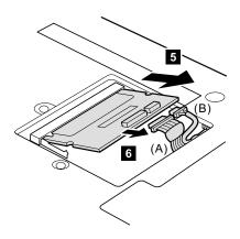
When installing: Make sure not to pinch the connector cable when re-installing the Mini PCI adapter.
