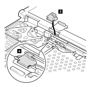
When installing: Make sure that the FPC bracket is firmly attached as shown in the figure **a**.
