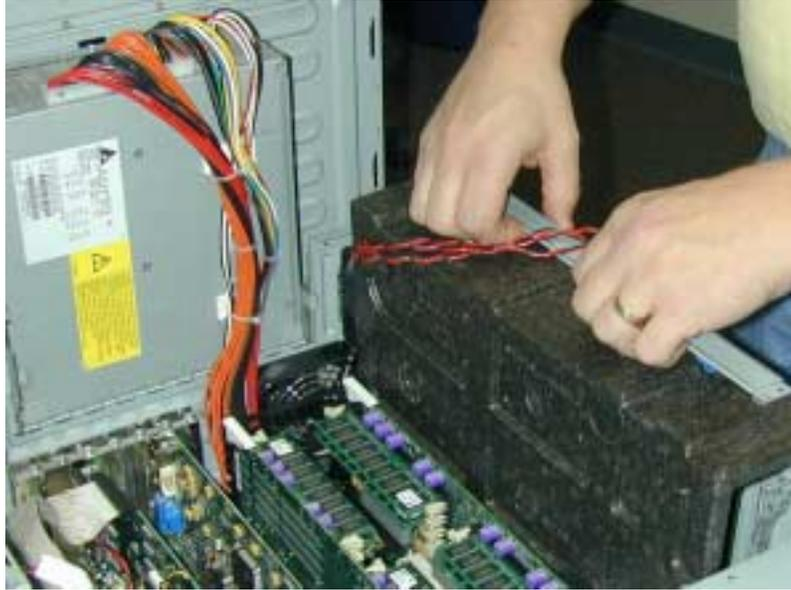
*Figure 5 Processor assembly*
