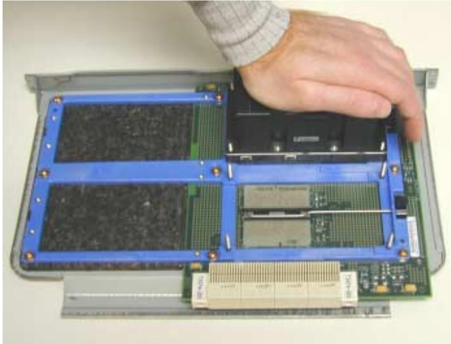
Figure 22 Properly seating the processor
