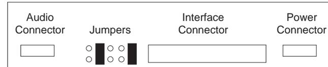
See “Connectors and settings for additional drives” on page 114 for information on setting and attaching IDE/AT interface drives.
