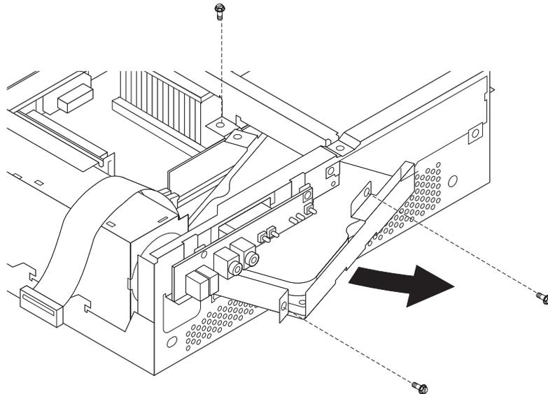
4. Disconnect all hard disk drive wires.
