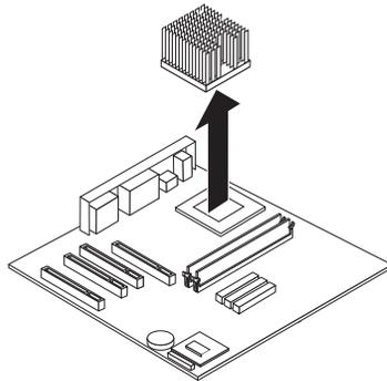
5. To remove the fansink from the processor, twist the fansink to break the seal formed by the thermal grease and remove.
