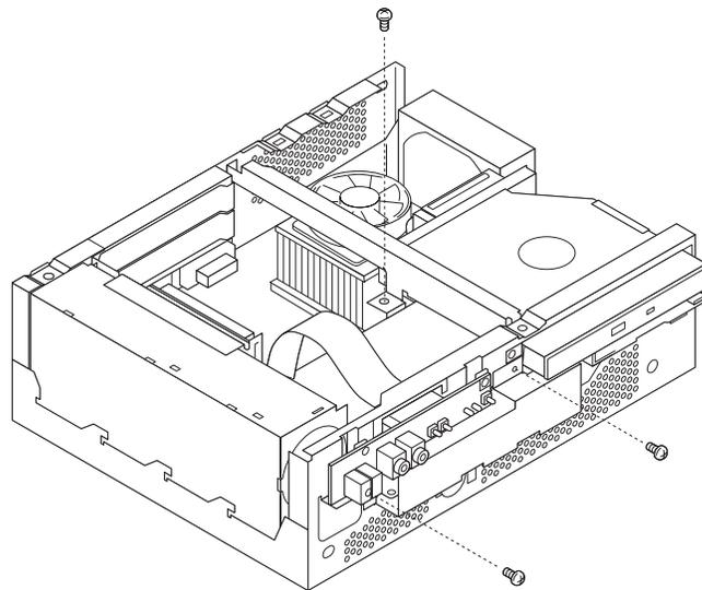
5. Unplug the flat cable attached to the small circuit board at the front.
