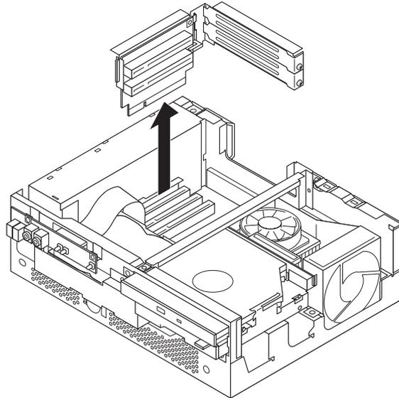
3. Remove the adapter-slot-cover latch and the slot cover for the appropriate expansion slot.
