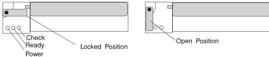
b. Position the drive carrier assembly horizontally, with the connector facing into the bay.
