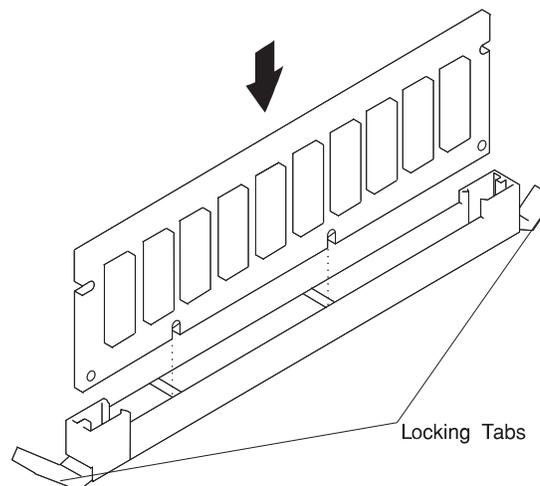
**Attention:** Inserting the memory-module kit diagonally may damage the memory-module kit.
