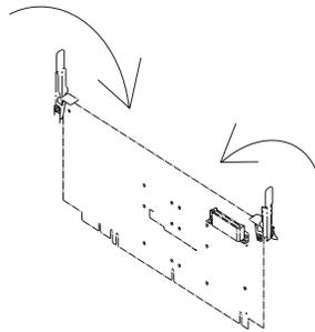
3. Connect the power cable to the CPU card.
