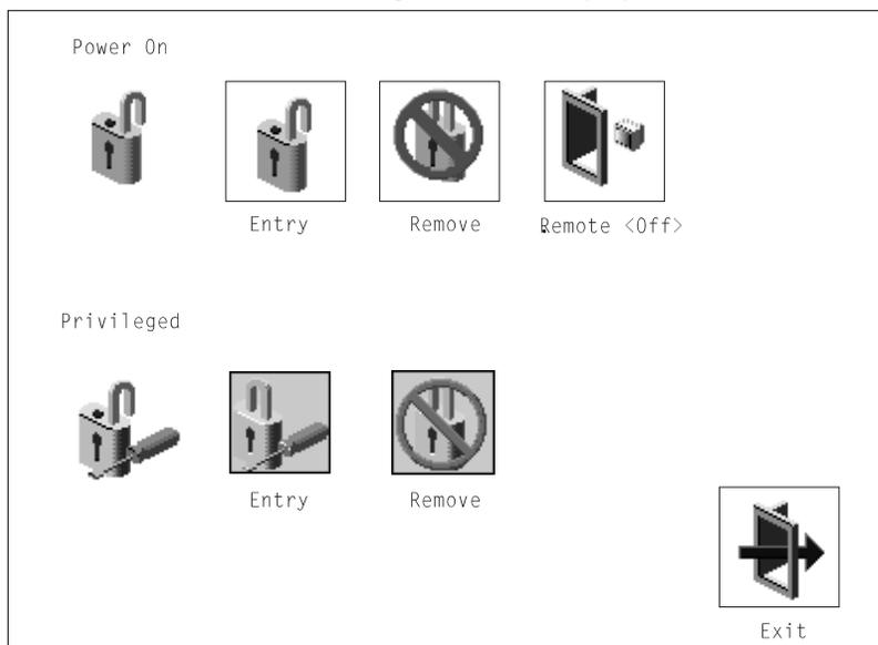
**Power-On Password:** Setting a power-on password helps protect information stored in your computer. If a power-on password is set for your computer, the Power On icon is shown in the locked position; if a power-on password is not set, then the Power On icon is shown in the unlocked position (as in the screen above).
