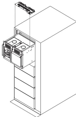
**Replacement:** Attach the new power distribution assembly to the bracket, and replace in reverse order.
