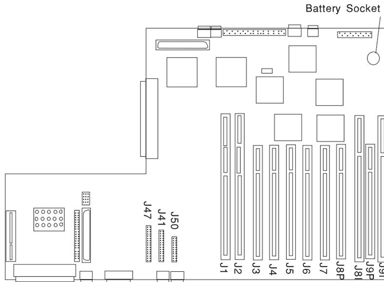
3. Use one finger to slightly slide the battery toward the front of the server. (The spring mechanism behind the battery will push it out toward you as you slide it forward.) Use your thumb and index finger to hold the battery as it pushes out of the socket.
