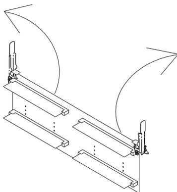
4. Carefully lift the memory card out of the slot.
