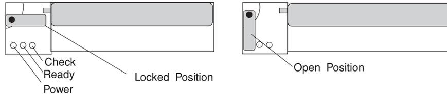
The following table explains the meaning of the Power, Ready and Check status LEDs on a SSA disk drive.
