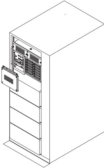
3. Each hot swap disk drive you plan to replace must have the hot swap SCSI disk drive carrier attached.
