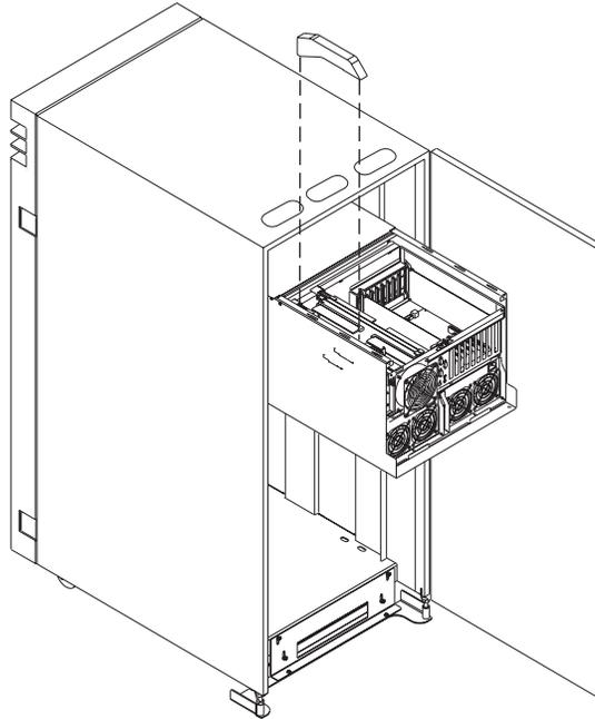
**Replacement:** To replace the CPU air flow duct, perform the removal steps in the reverse order.
