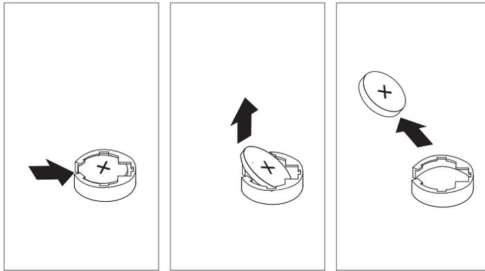
**Replacement:** Tilt the battery so that you can insert it into the front of the socket. As you slide the battery toward the front of the server, push it down into the socket.
