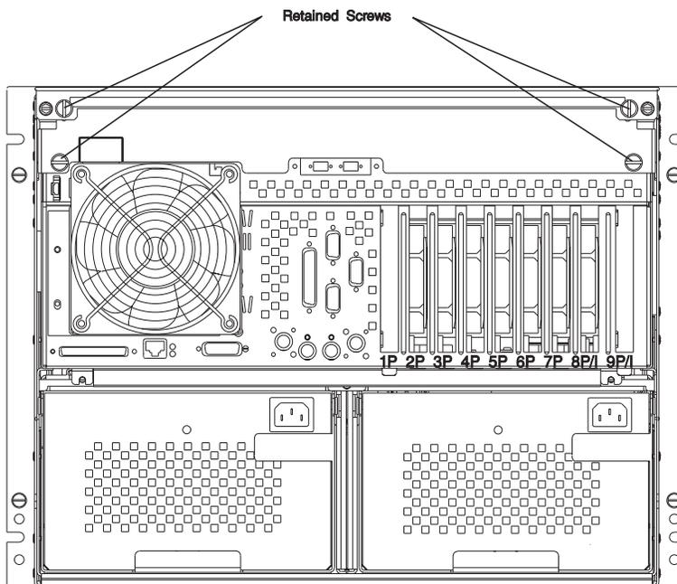
14. Loosen the lower two retained screws (one on each side) and slide the cover to the rear to remove the inner rear access cover.
