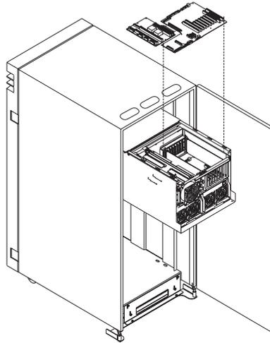
14. Disconnect the system board from the I/O board.
