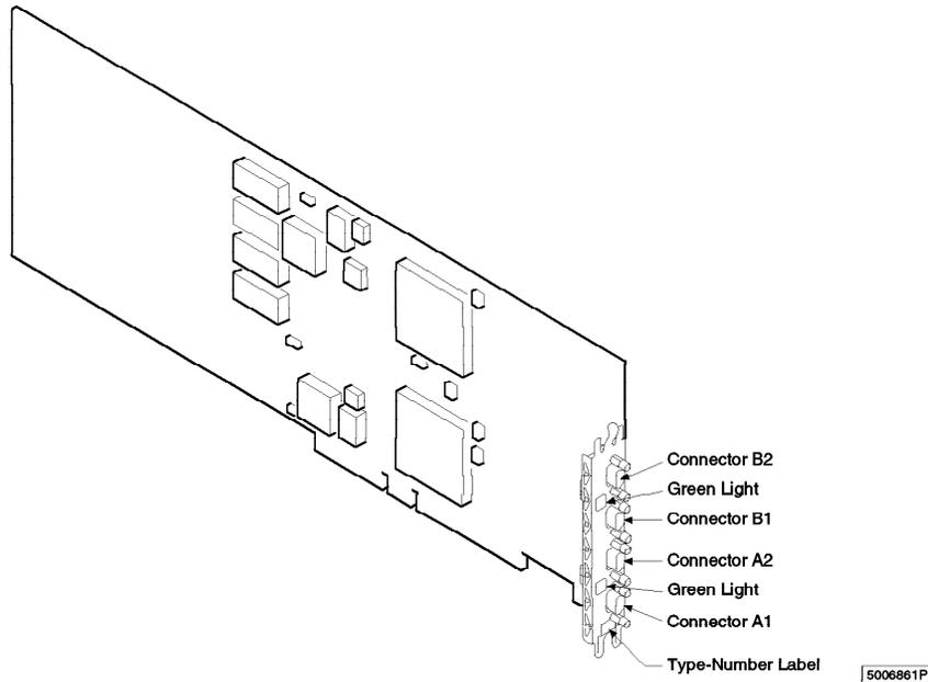
The SSA links must be configured as loops. The loop is connected to the internal connectors at the SSA adapter card. These connectors *must* be a valid pair (that is, A1 and A2, or B1 and B2); otherwise, the disk drive modules on the loop are not fully configured, and the diagnostics fail. Operations to all the disk drive modules on a particular loop can continue if that loop breaks at any one point.
