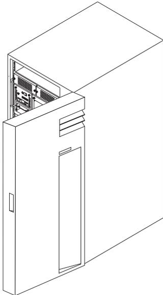
2. Loosen the screws that hold the disk drive cover to the drawer and remove the the disk drive cover from the drawer, storing it in a safe place.
