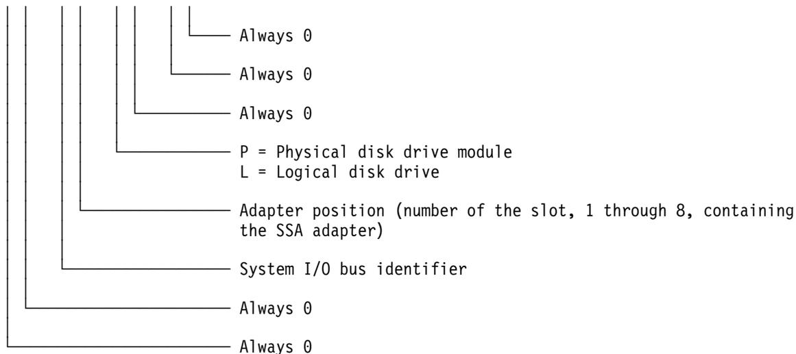
The location code shows only the position of the SSA adapter in the using system and the type of device that is attached. Use a service aid to find the location of the device (disk drive module). For more information, see "Using the Service Aids" in *RS/6000 Enterprise Server Model H50 User's Guide*.
