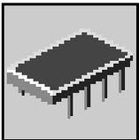
**Memory Test:** CHRP systems have a memory test option available. The memory test runs patterns thru memory and check the results. This is a pass/fail test. If the test fails, the failure is noted in the error log and displayed on the utilities menu screen.
