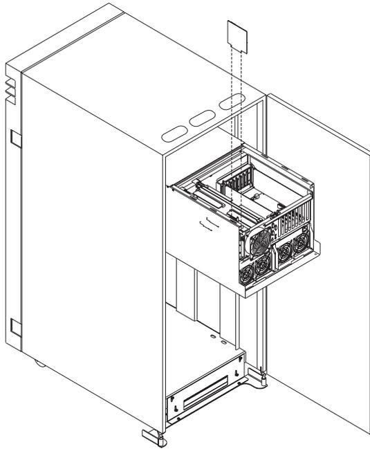
**Replacement:** To replace the service processor card, perform the removal steps in the reverse order.
