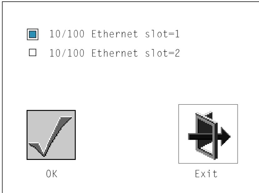
The next screen allows you to select the configuration of the adapter you have just chosen (or allow the system to select the configuration automatically). As on the previous screen, use the arrow keys to highlight, press the space bar to select, then highlight the OK icon and press enter.
