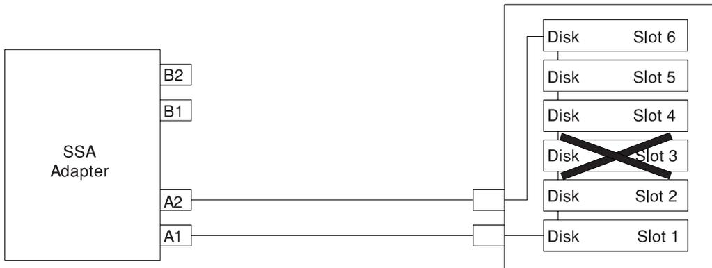
If two or more disk drive modules are turned off, fail, or are removed from the loop, some modules might become isolated from the SSA adapter.
