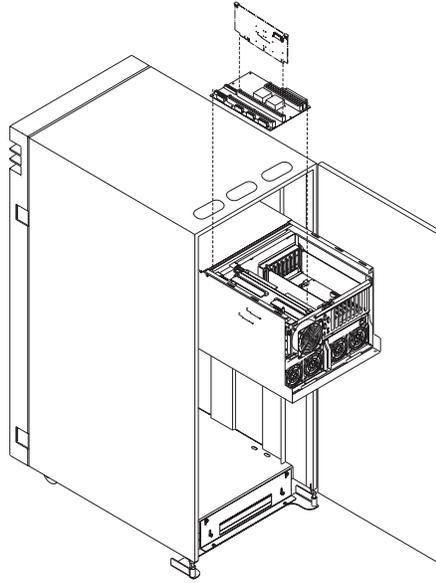
**Replacement:** To replace the CPU Card, perform the removal steps in the reverse order.
