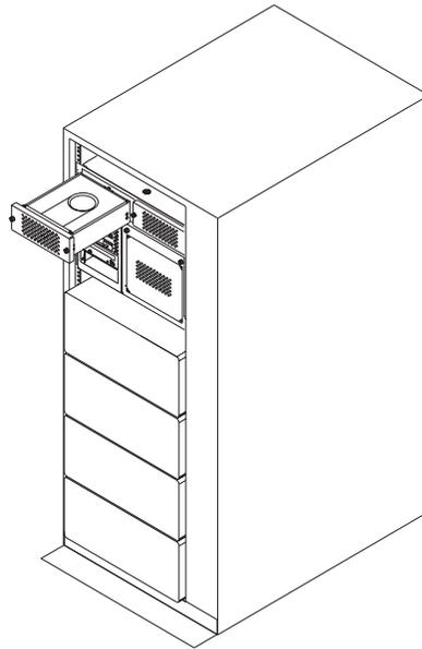
**Replacement:** Replace in reverse order. Ensure that the retained screws are properly engaged, as they draw the blower assembly into the blower connectors.
