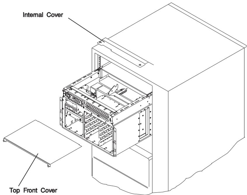
4. Remove the internal cover by loosening the two thumbscrews.
