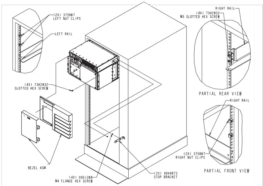
3. Lift the I/O Drawer onto the support rails, and slide it **slowly** into the rack until the first hexhead flange screw. Slip the angled end of each chassis stop bracket behind the rack frame and position the slotted clearance holes over the hexhead flange screws. Tighten the hexhead flange screws securely.
