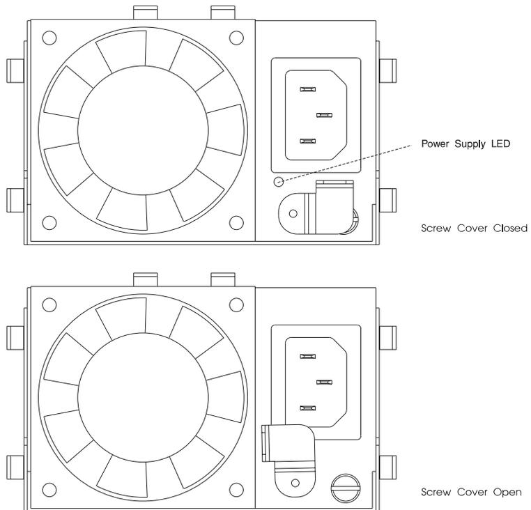
5. Plug the power cord into the power supply.
