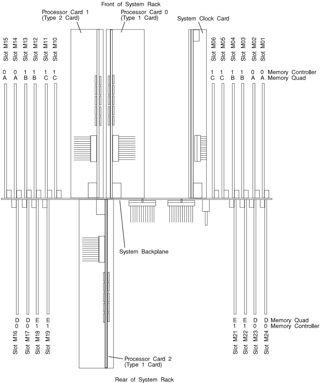
R1 Memory Cards are the primary memory cards used in the S70. All S70 memory cards are installed in four card functional units called quads. The quads must be composed of the four cards of the same type. The complete set of four cards must be properly installed in the proper card slots for the newly installed memory to work. See the figure on page 1-20 for the location of the card slots that are in each quad.
