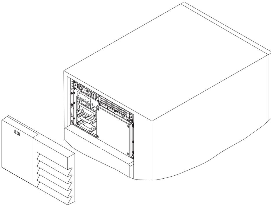
2. Remove the screws that hold the disk drive cover to the drawer and remove the disk drive cover from the drawer, storing it in a safe place.
