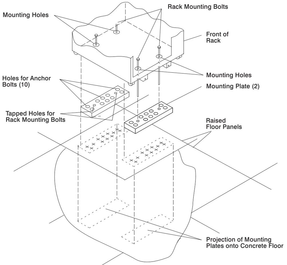
9. At the marked location of the tapped mounting holes, drill two holes approximately 1 inch to allow clearance for the ends of the two rack-mounting bolts (the
