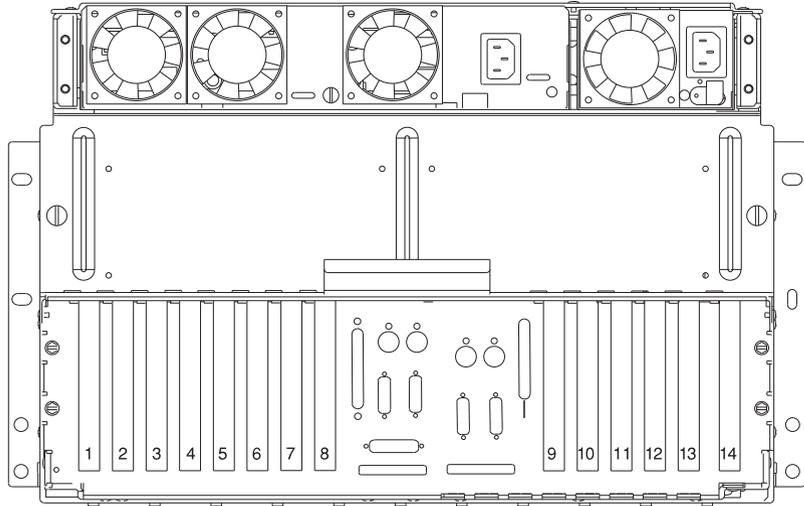
3. Remove the acoustic baffle from the rear of the I/O Drawer, as described in “Acoustic Baffle” on page 9-34.
