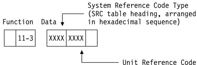
Figure 6-1. Determining the SRC and URC
