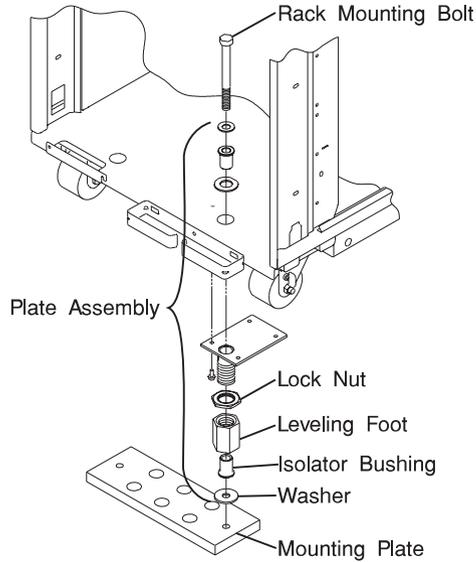
2. Place the mounting plates, front and rear, (note they are different) in the approximate mounting position under the System Rack.
