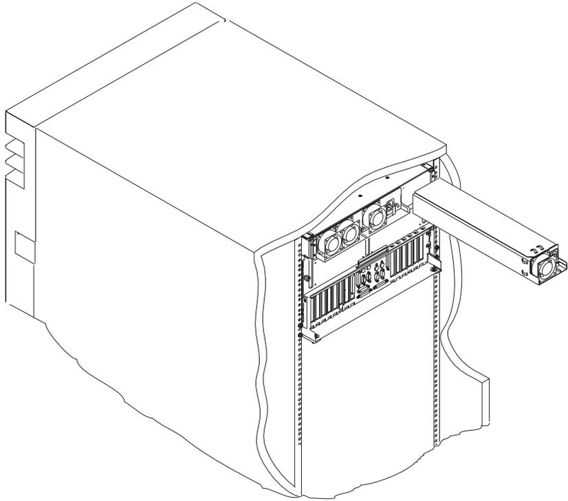
7. To remove the 3/4 power supply, slide the screw cover to the left to the open position to access the power supply screw.
