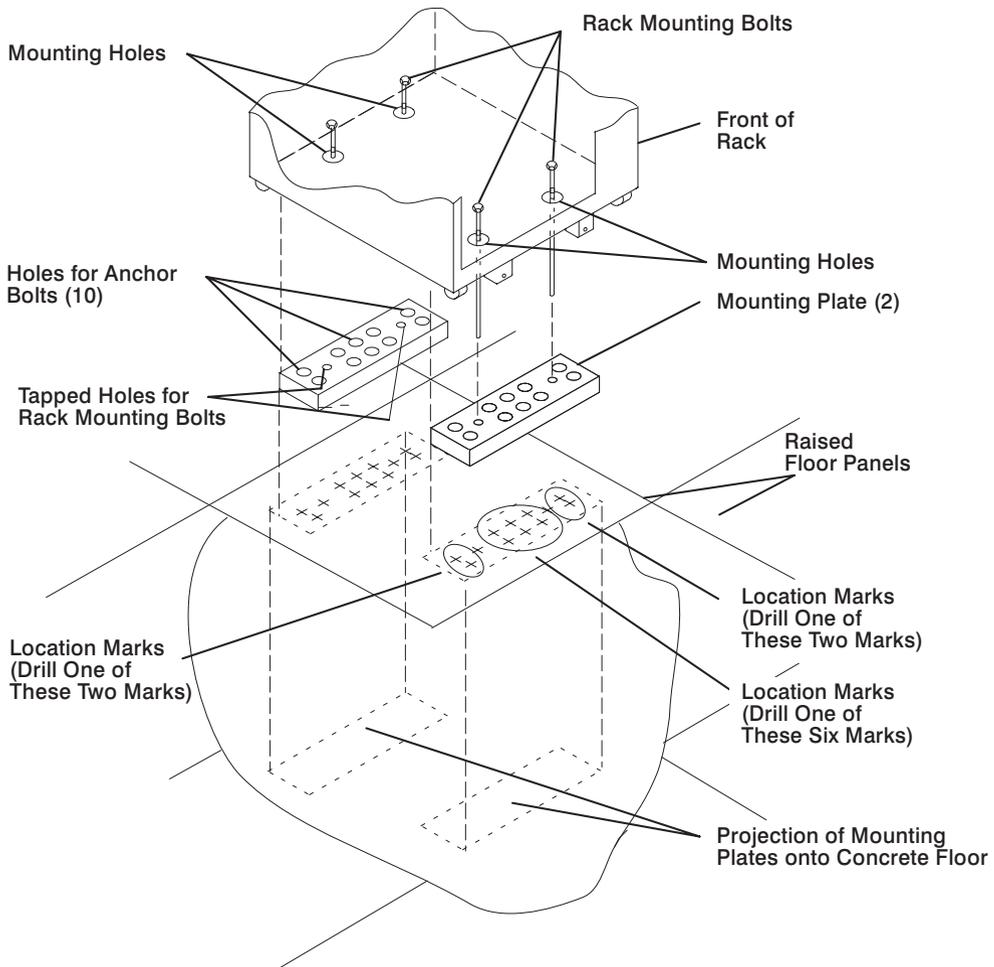
13. Place the two mounting plates on the locations indicated on the marked raised-floor panel.
