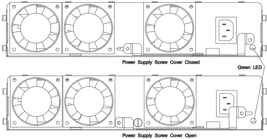
10. Plug the power cord into the power supply.
