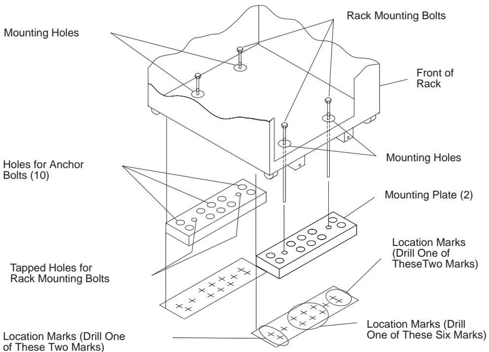
10. Drill one hole in each group of anchor bolt location marks as indicated on the marked floor.
