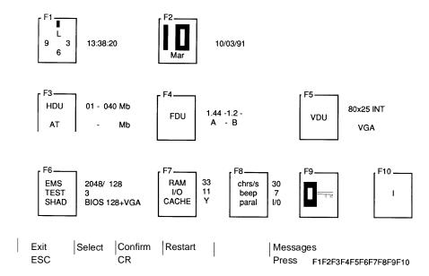
This menu includes all icons of the BUILT IN SETUP and allows the system to be configured as described previously.
