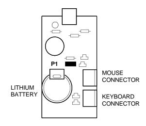
P1 inserted: Battery enabled, data in the CMOS RAM
