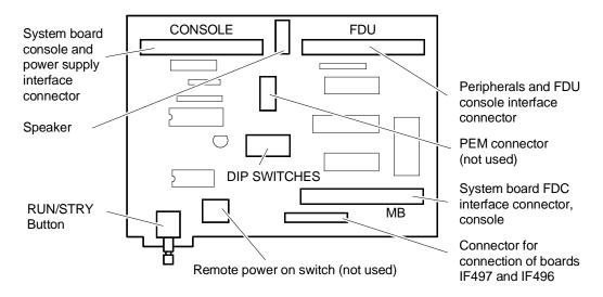
**DIP-SWITCHES** for the configuration of peripherals with floppy disk interface
