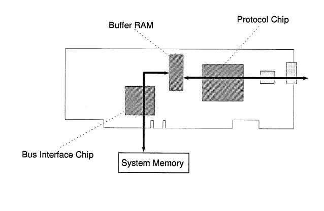
**Figure 2. Store and Forward Busmaster Adapter.** The system CPU is only used to initiate data transfers. The adapter must buffer the entire frame.
