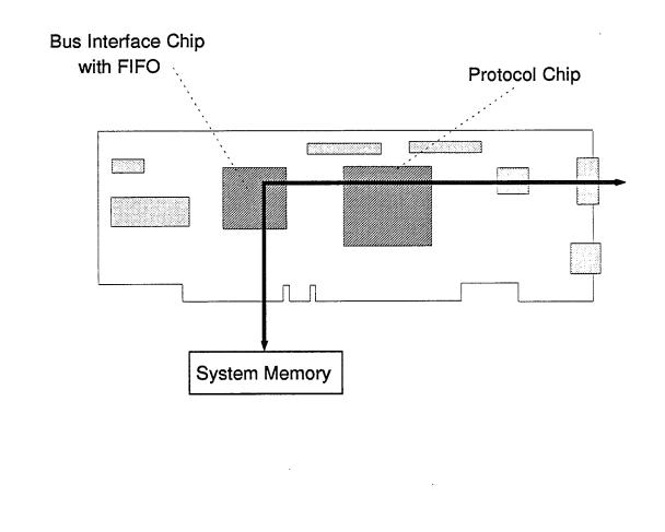
**Figure 3. LANStreamer Adapter.** The adapter has no buffer memory. Frames are transferred directly between the LAN and system memory.
