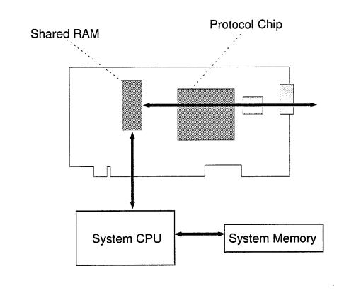
**Figure 1. Shared RAM Adapter.** The system CPU is involved in the transfer of each and every byte of every frame.
