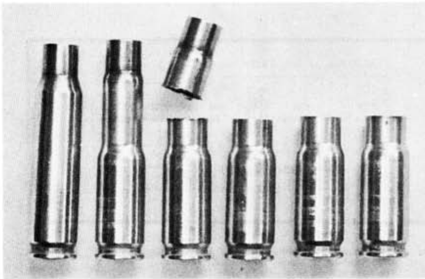
This sequence illustrates the steps necessary to form .357 AMP cases from 7.62mm NATO brass. The case is first run into a form/trim die, the excess is sawed off, then the case is trimmed, neck reamed, resized, and the case mouth is flared. The sectioned cases above, from left, are the trimmed and reamed 7.62mm NATO formed to .44 AMP, and CDM .44; both are suitable for forming to .357 AMP, right.
