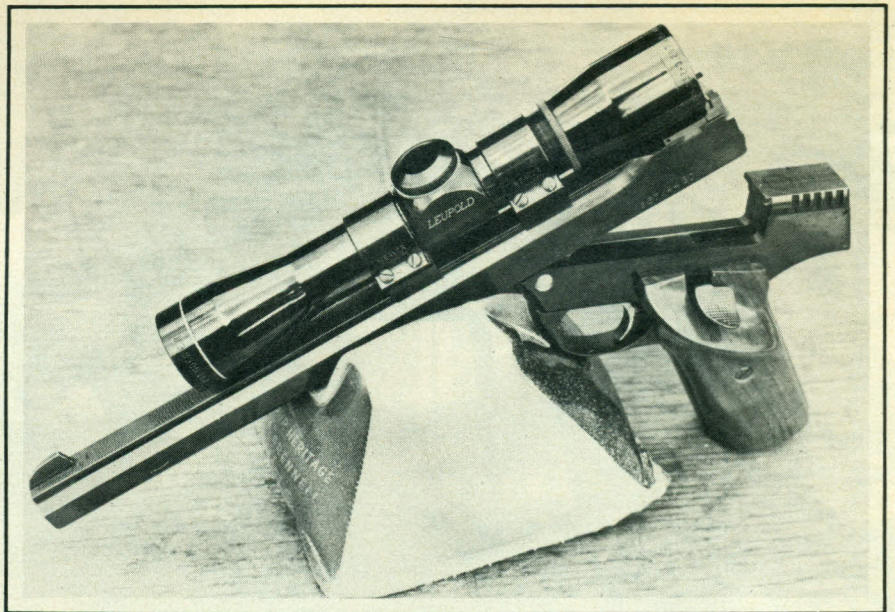
Merrill barrels are changed by removing pivot bolt. Catch at top rear of receiver is pulled rearward to open breech. Safety latch, visible here above thumb rest, must be pushed down in order to fire. Action cocks on opening.
