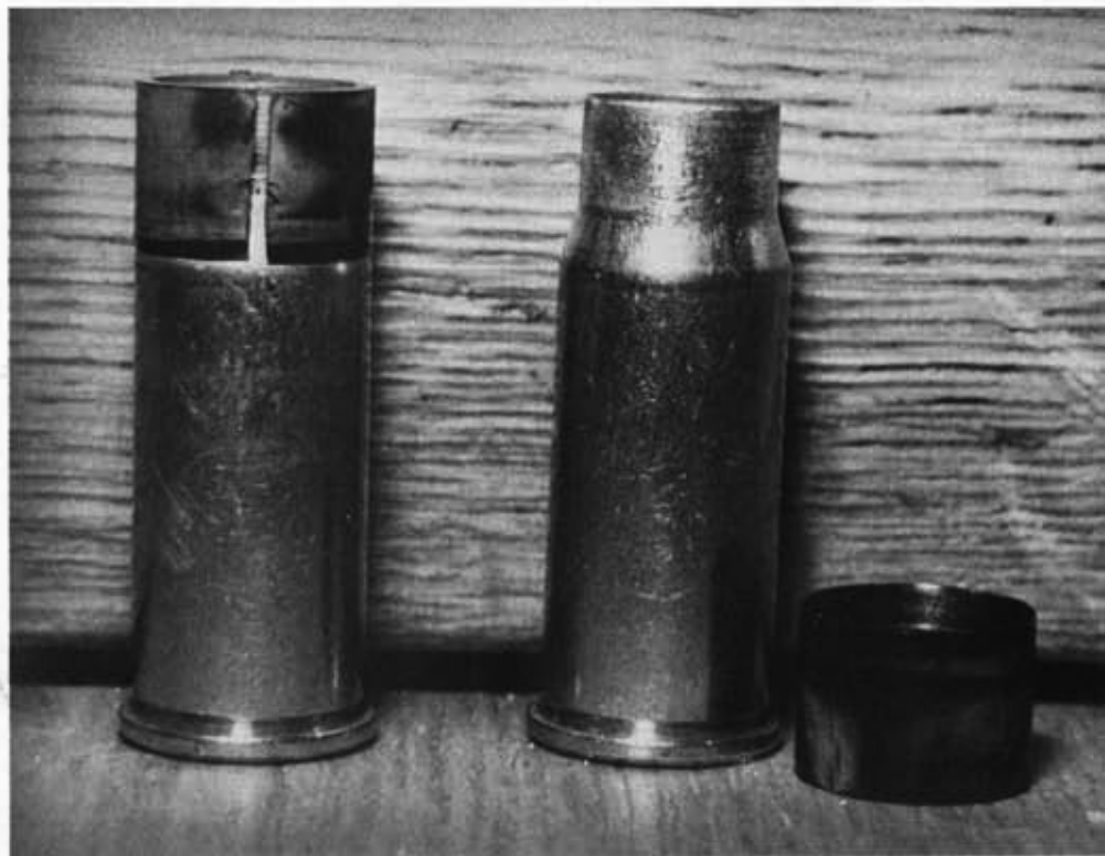
Though the plastic collars on the neck of the Bobcat often split upon firing, it has no effect on performance, being designed for one-time use.
