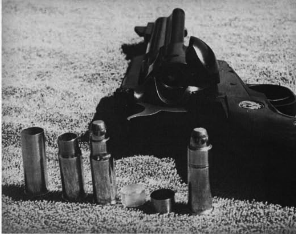
Progression of the conversion shows .44 Magnum case (left); a necked case; a loaded round; the collars and a complete round ready to go.
