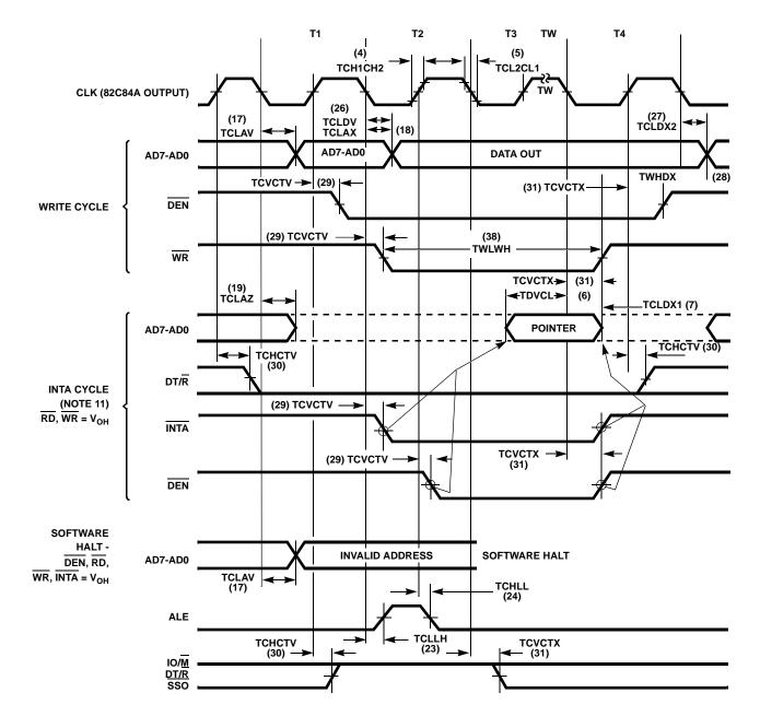
FIGURE 11. BUS TIMING - MINIMUM MODE SYSTEM (Continued)
