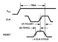
FIGURE 18. RESET TIMING
