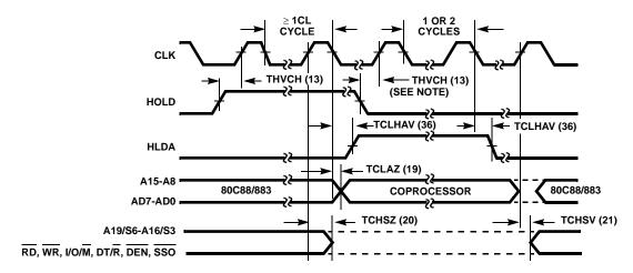
FIGURE 15. HOLD/HOLD ACKNOWLEDGE TIMING (MINIMUM MODE ONLY)
