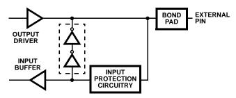
FIGURE 6. BUS HOLD CIRCUITRY PINS 2-16 AND 35-39
