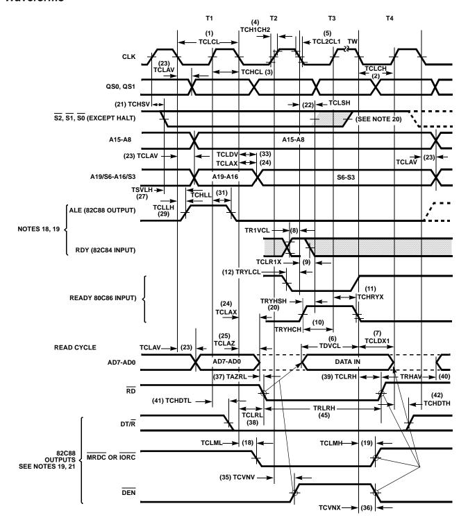
FIGURE 12. BUS TIMING - MAXIMUM MODE (USING 82C88)
