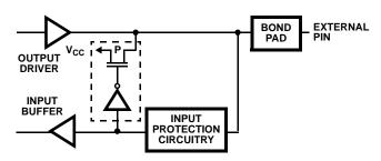
FIGURE 7. BUS HOLD CIRCUITRY PINS 26-32 AND 34
