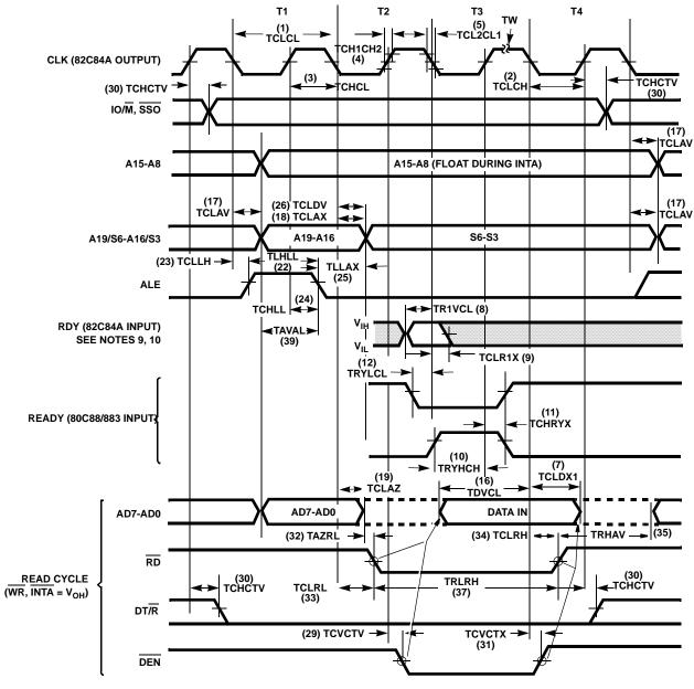
FIGURE 10. BUS TIMING - MINIMUM MODE SYSTEM
