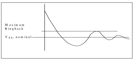
Figure 14-2. Maximum Ringback Associated with the Signal Low State
