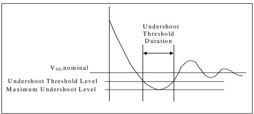
Figure14-1. Maximum Undershoot Level, Undershoot Threshold Level, and Undershoot
