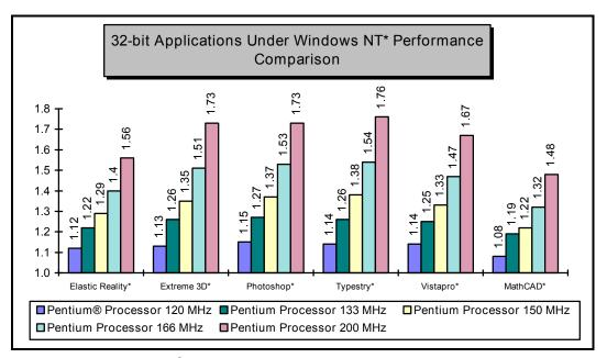
Figure 10. Intel Pentium <sup>®</sup> Processor Performance for 32-bit Applications Under Windows NT\* (Scaled to the Pentium Processor at 100 MHz)
