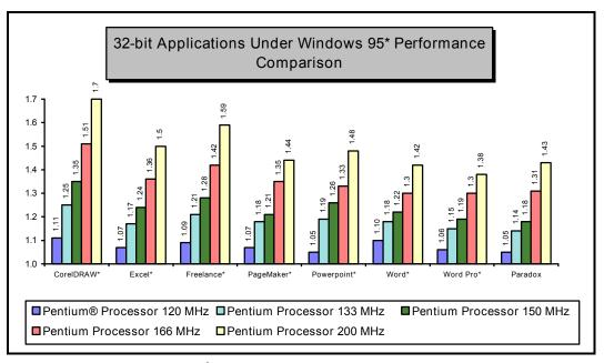
Figure 11. Intel Pentium \* Processor Performance for 32-bit Applications Under Windows 95\* (Scaled to the Pentium Processor 100 MHz)
