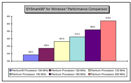
Figure 8. Intel Pentium Processor Performance for the SYSmark95\* for Windows for Workgroups\* Benchmark
