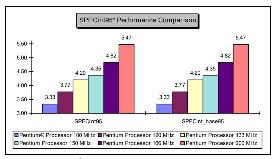
Figure 2. Intel Pentium <sup>®</sup> Processor Performance for the UNIX\* SPECint95\* Benchmark with 1 MB L2 Cache on Pentium Processors at 100, 120, 133, 150, 166 and 200 MHz
