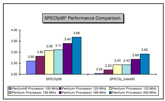
Figure 3. Intel Pentium <sup>®</sup> Processor Performance for the UNIX\* SPECfp95\* Benchmark with 1 MB L2 Cache on Pentium Processors at 100, 120, 133, 150, 166 and 200 MHz
