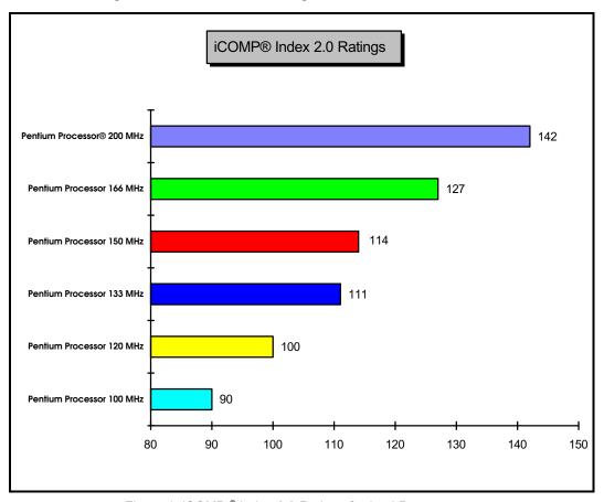
Figure 1. iCOMP <sup>®</sup> Index 2.0 Ratings for Intel Processors (System configurations are listed in Appendix A.)
