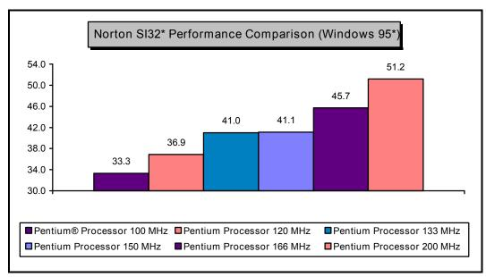
Figure 4. Intel Pentium ® Processor Performance for the Norton SI32\* Benchmark
