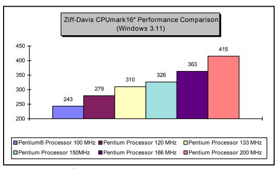
Figure 7. Intel Pentium <sup>®</sup> Processor Performance for the Ziff-Davis CPUmark16\* Benchmark
