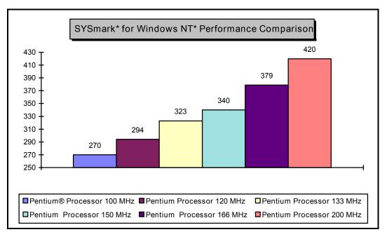
Figure 9. Intel Pentium \* Processor Performance for SYSmark\* for Windows NT\*
