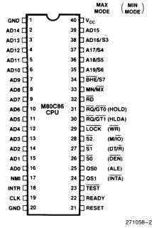
Figure 2. M80C86 40-Lead DIP Configuration
