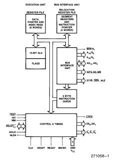
Figure 1. M80C86 CPU Block Diagram
