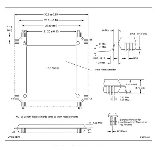
Figure 14. 208-Lead SQFP Package Dimensions
