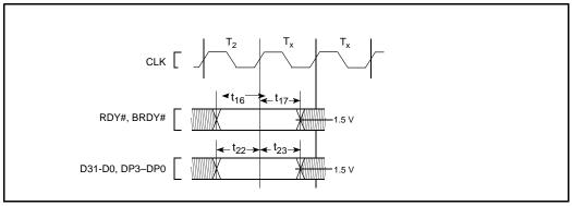
Figure 6. Input Setup and Hold Timing
