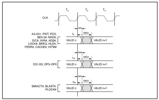
Figure 8. Output Valid Delay Timing
