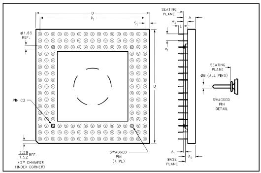
Figure 15. Principal Dimensions and Data for 168-Pin Pin Grid Array Package
