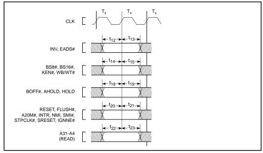
Figure 5. Input Setup and Hold Timing
