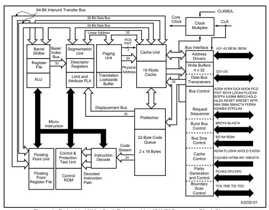
Figure 1. Embedded Write-Back Enhanced IntelDX4™ Processor Block Diagram
