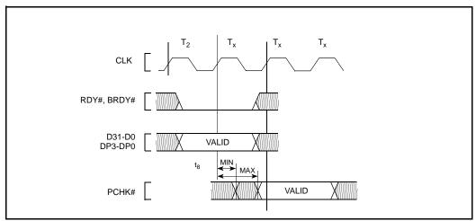
Figure 7. PCHK# Valid Delay Timing
