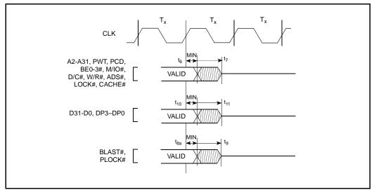
Figure 9. Maximum Float Delay Timing
