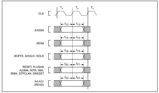
Figure 10. Input Setup and Hold Timing
