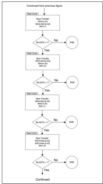
Figure 7. Address Prediction for Burst Transfers (2 of 3)
