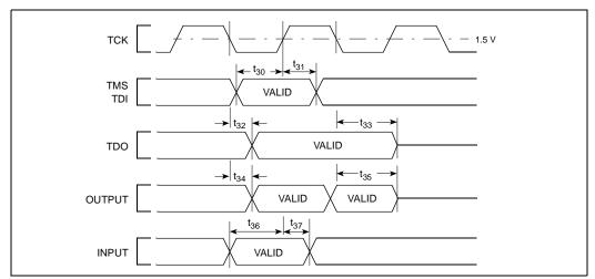
Figure 16. Test Signal Timing Diagram
