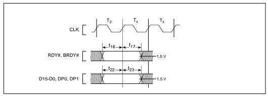
Figure 11. Input Setup and Hold Timing
