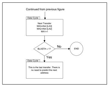
Figure 8. Address Prediction for Burst Transfers (3 of 3)
