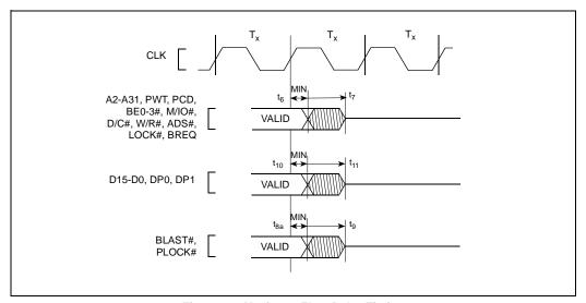
Figure 14. Maximum Float Delay Timing
