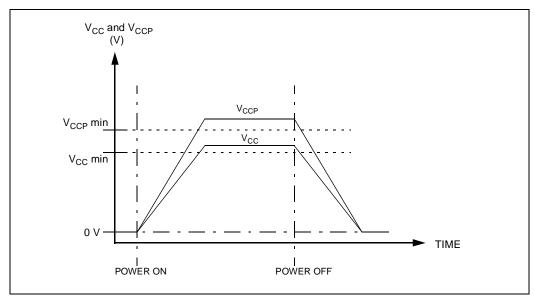
Figure 3. Example of Supply Voltage Power Sequence
