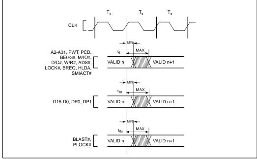
Figure 12. Output Valid Delay Timing
