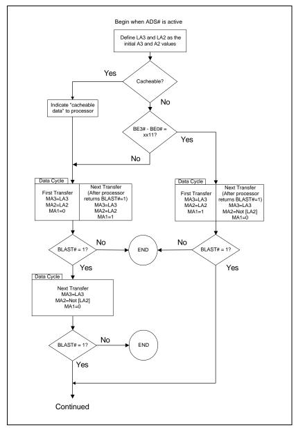
Figure 6. Address Prediction for Burst Transfers (1 of 3)
