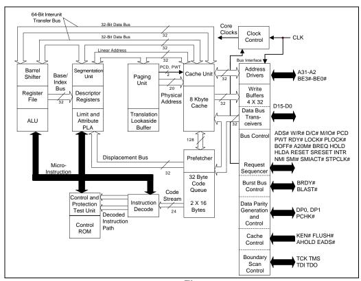
Figure 1. Embedded ULP Intel486<sup>TM</sup> GX Processor Block Diagram
