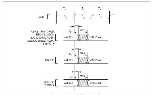
Figure 8. Output Valid Delay Timing
