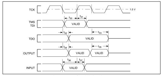
Figure 11. Test Signal Timing Diagram
