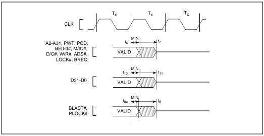
Figure 9. Maximum Float Delay Timing
