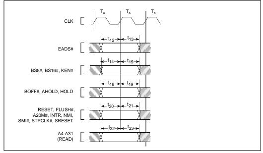
Figure 6. Input Setup and Hold Timing
