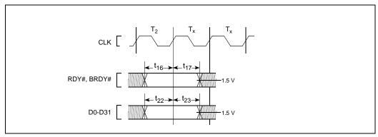
Figure 7. Input Setup and Hold Timing
