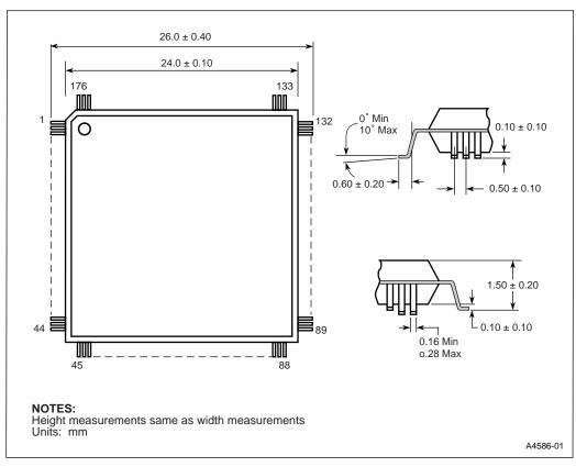
Figure 14. Package Mechanical Specifications for the 176-Lead TQFP Package
