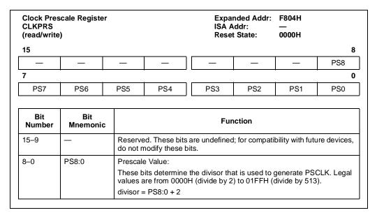
Figure 13-17. Clock Prescale Register (CLKPRS)
