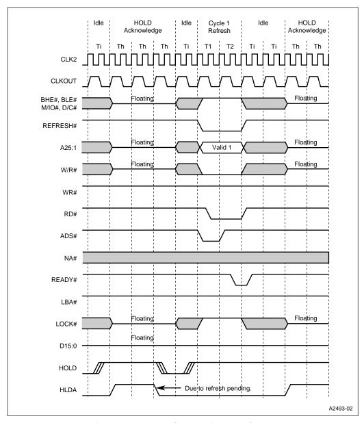
Figure 6-12. Refresh Cycle During HOLD/HLDA
