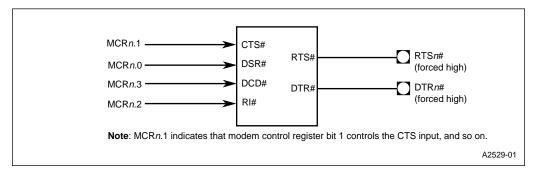
Figure 11-19. Modem Control Signals - Diagnostic Mode Connections
