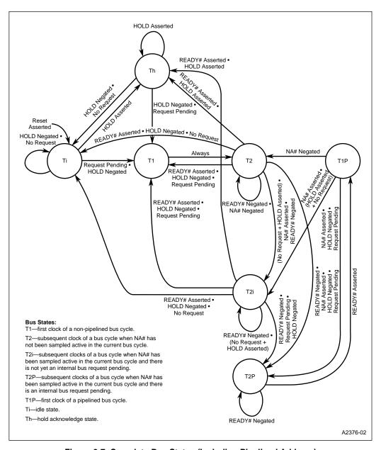
Figure 6-7. Complete Bus States (Including Pipelined Address)
