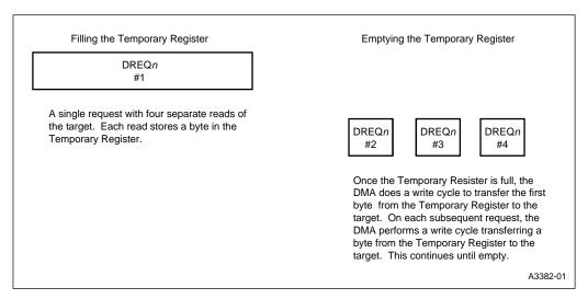
Figure 12-3. DMA Temporary Buffer Operation for A Write Transfer
