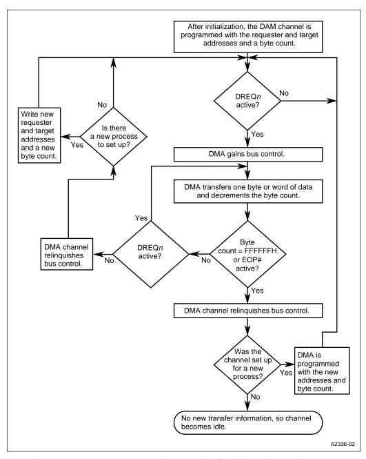
Figure 12-16. Demand Data-transfer Mode with Chaining Buffer-transfer Mode
