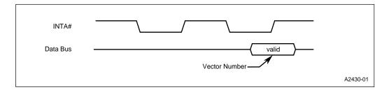
Figure 9-17. Interrupt Acknowledge Cycle
