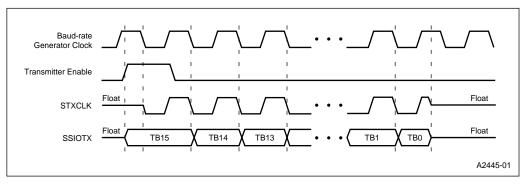
Figure 13-10. Transmitter Master Mode, Single Word Transfer (Enabled when Clock is High)
