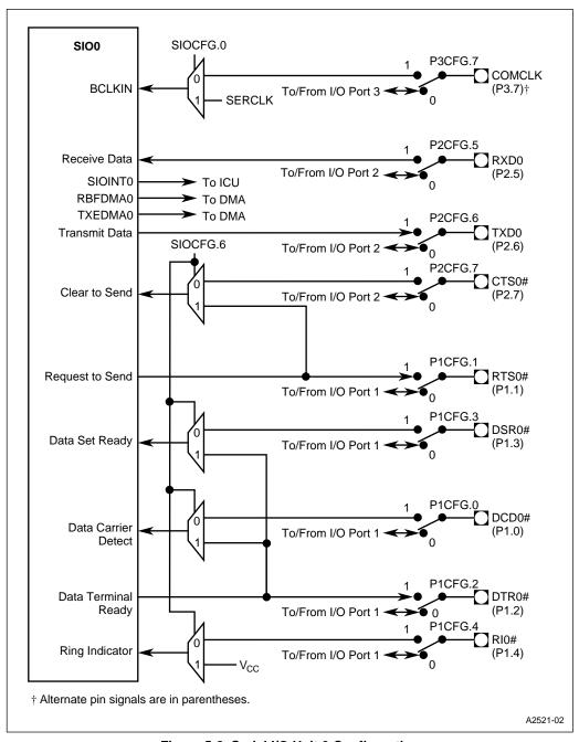
Figure 5-8. Serial I/O Unit 0 Configuration
