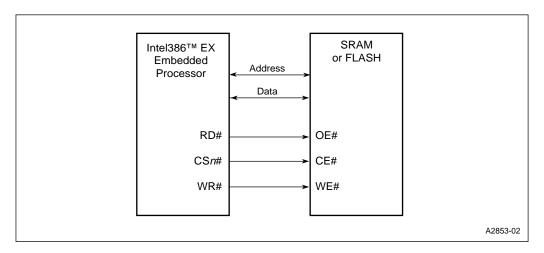
Figure 6-16. Intel386 EX Processor to SRAM/FLASH Interface
