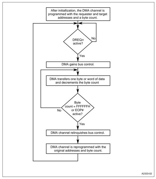
Figure 12-12. Block Data-transfer Mode with Autoinitialize Buffer-transfer Mode
