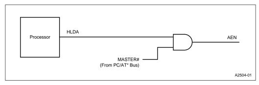
Figure B-1. Derivation of AEN Signal in a Typical PC/AT System
