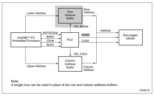
Figure 6-19. Intel386 EX Processor and Non-Paged DRAM Interface
