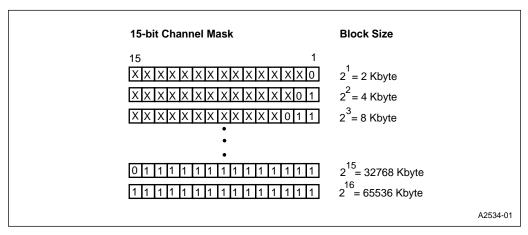
Figure 14-2. Determining a Channel's Address Block Size
