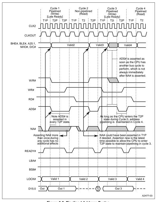
Figure 6-8. Pipelined Address Cycles
