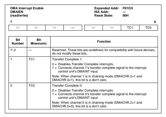
Figure 12-33. DMA Interrupt Enable Register (DMAIEN)
