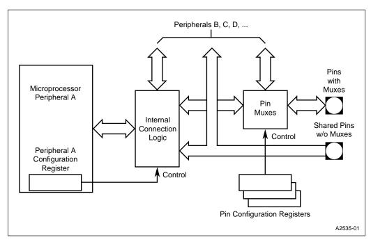
Figure 5-1. Peripheral and Pin Connections
