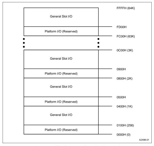
Figure 4-1. PC/AT I/O Address Space (10-bit Decode)
