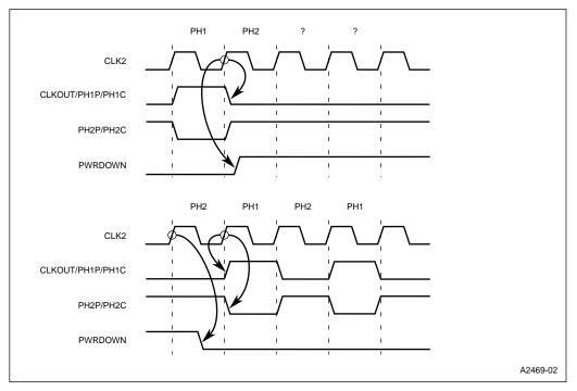
Figure 8-7. Timing Diagram, Entering and Leaving Powerdown Mode
