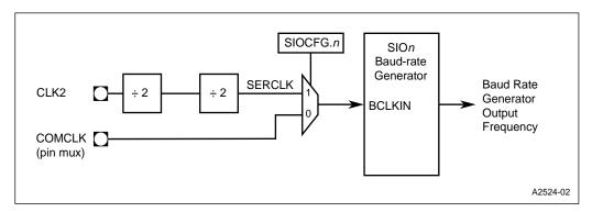
Figure 11-2. SIOn Baud-rate Generator Clock Sources
