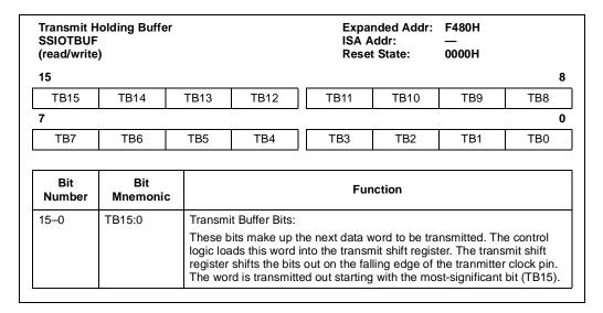
Figure 13-22. SSIO Transmit Holding Buffer (SSIOTBUF)
