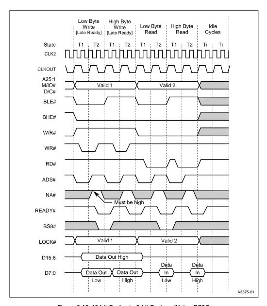
Figure 6-13. 16-bit Cycles to 8-bit Devices (Using BS8#)
