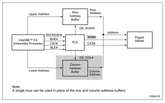
Figure 6-18. Intel386 EX Processor to Paged DRAM Interface
