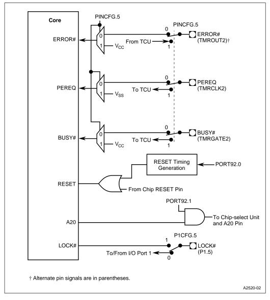
Figure 5-13. Core Configuration
