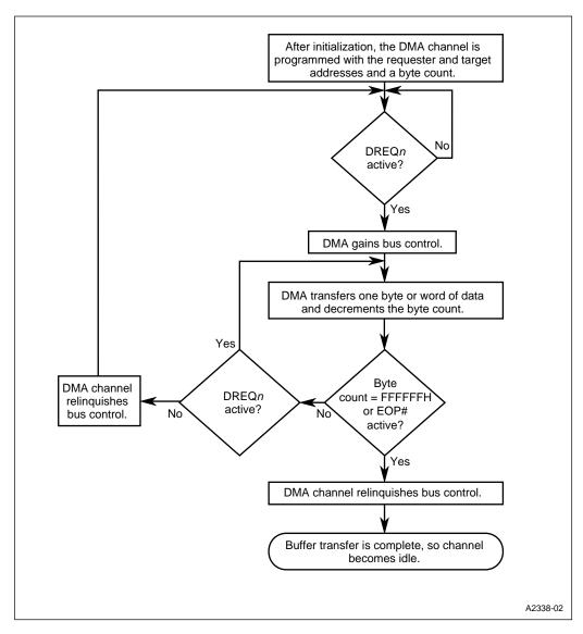
Figure 12-14. Demand Data-transfer Mode with Single Buffer-transfer Mode
