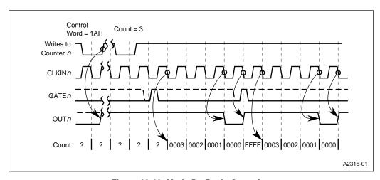
Figure 10-19. Mode 5 - Basic Operation
