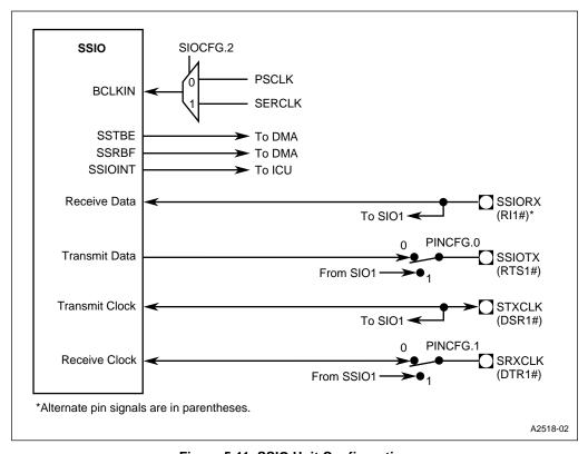
Figure 5-11. SSIO Unit Configuration
