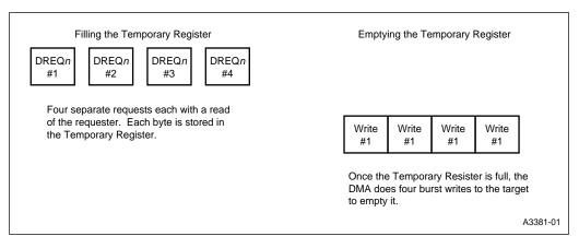
Figure 12-2. DMA Temporary Buffer Operation for a Read Transfer
