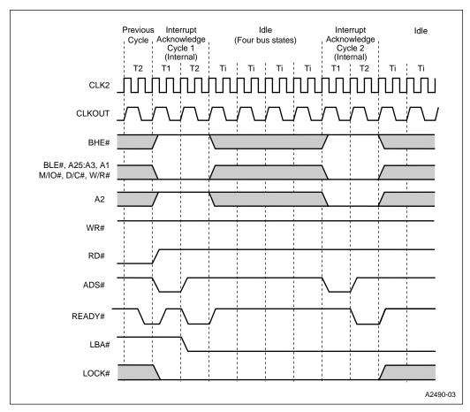
Figure 6-9. Interrupt Acknowledge Cycles
