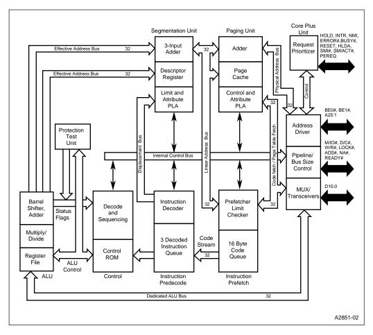
Figure 3-2. The Intel386™ CX Processor Internal Block Diagram
