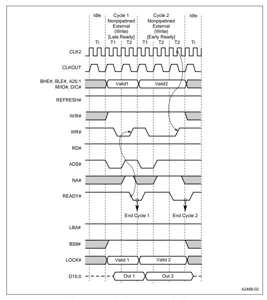
Figure 6-6. Nonpipelined Address Write Cycles
