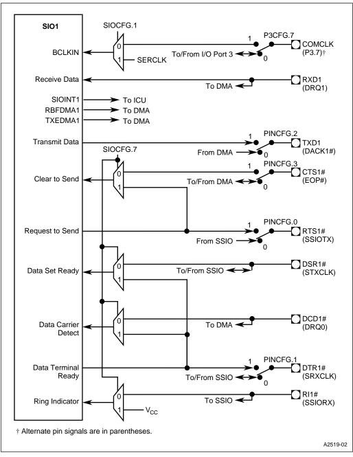
Figure 5-9. Serial I/O Unit 1 Configuration
