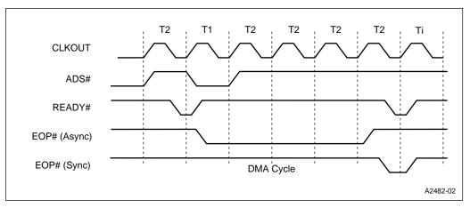
Figure 12-7. Buffer Transfer Ended by the EOP# Input
