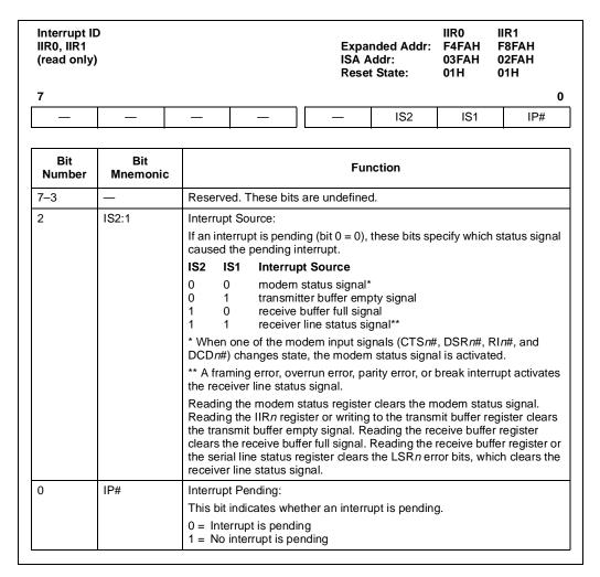
Figure 11-18. Interrupt ID Register (IIRn)
