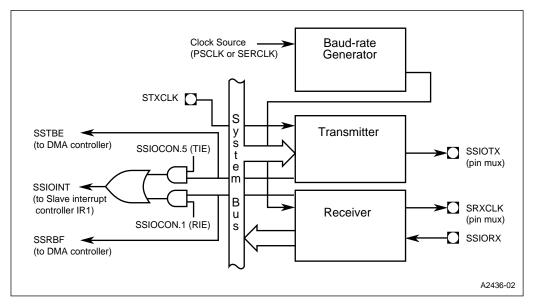
Figure 13-3. Transmitter in Slave Mode, Receiver in Master Mode
