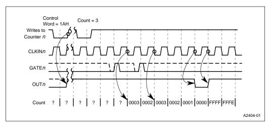
Figure 10-20. Mode 5 - Retriggering the Strobe
