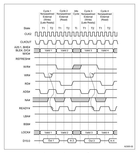
Figure 6-1. Basic External Bus Cycles
