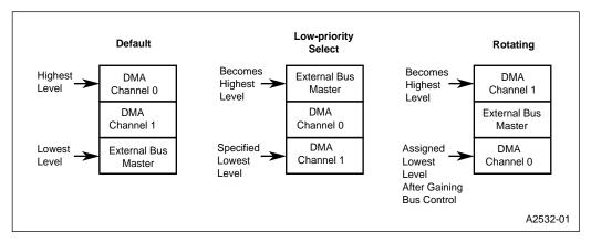
Figure 12-5. Changing the Priority of the DMA Channel and External Bus Requests
