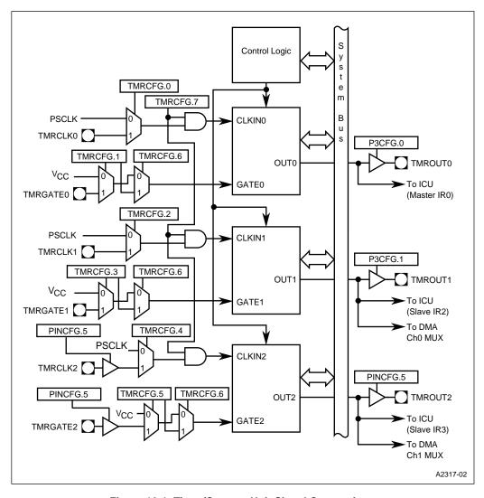
Figure 10-1. Timer/Counter Unit Signal Connections
