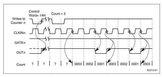
Figure 10-8. Mode 2 - Basic Operation
