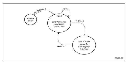
Figure 13-6. SSIO Transmitter with Autotransmit Mode Enabled
