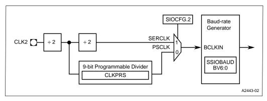
Figure 13-5. Clock Sources for the Baud-rate Generator
