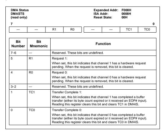
Figure 12-23. DMA Status Register (DMASTS)
