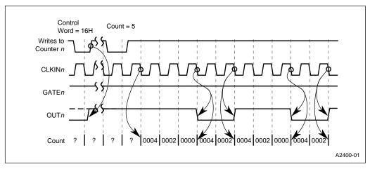
Figure 10-12. Mode 3 – Basic Operation (Odd Count)
