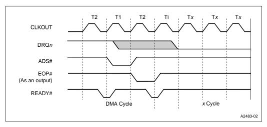
Figure 12-6. Buffer Transfer Ended by an Expired Byte Count
