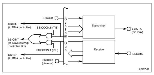
Figure 13-4. Transmitter and Receiver in Slave Mode
