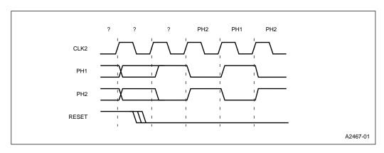
Figure 8-2. Clock Synchronization
