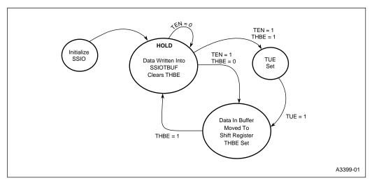
Figure 13-7. SSIO Transmitter with Autotransmit Mode Disabled
