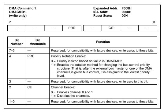
Figure 12-22. DMA Command 1 Register (DMACMD1)
