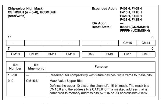
Figure 14-8. Chip-select High Mask Registers (CSnMSKH, UCSMSKH)
