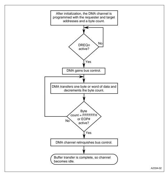
Figure 12-11. Block Data-transfer Mode with Single Buffer-transfer Mode
