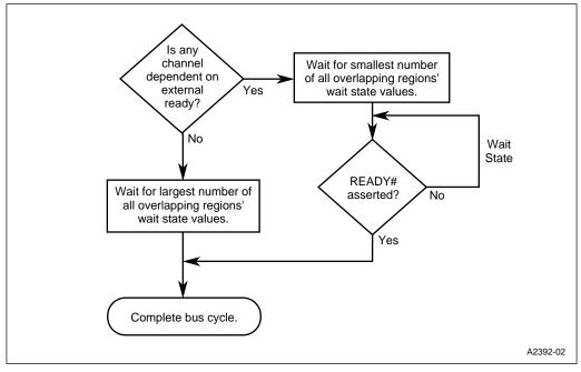
Figure 14-3. Bus Cycle Length Adjustments for Overlapping Regions
