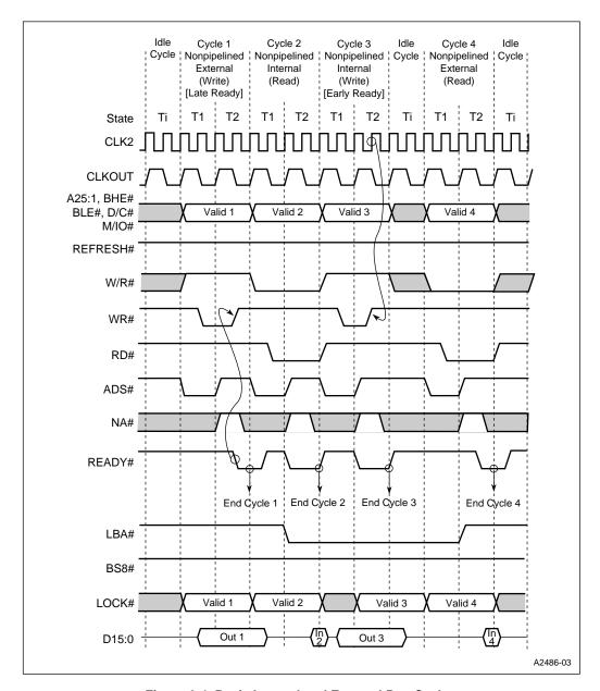
Figure 6-4. Basic Internal and External Bus Cycles
