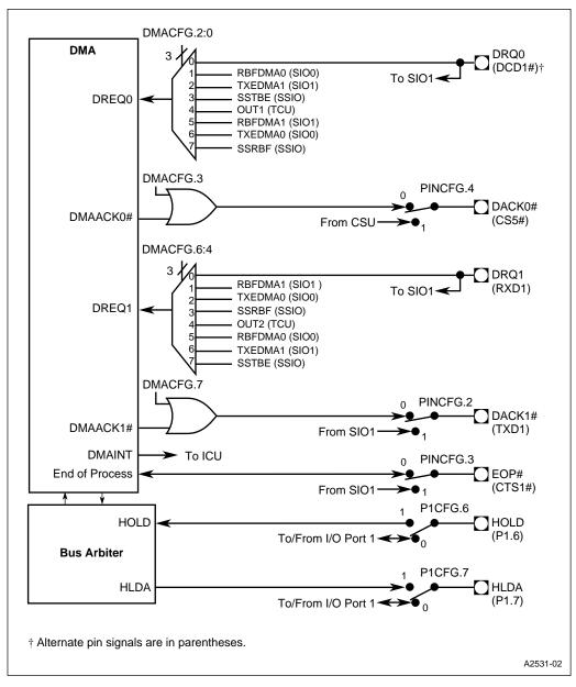
Figure 12-1. DMA Unit Block Diagram
