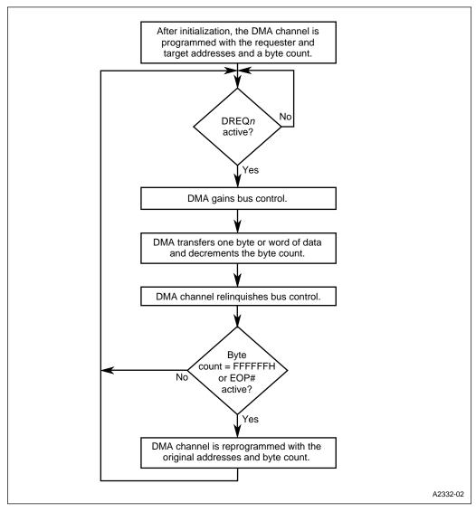
Figure 12-9. Single Data-transfer Mode with Autoinitialize Buffer-transfer Mode
