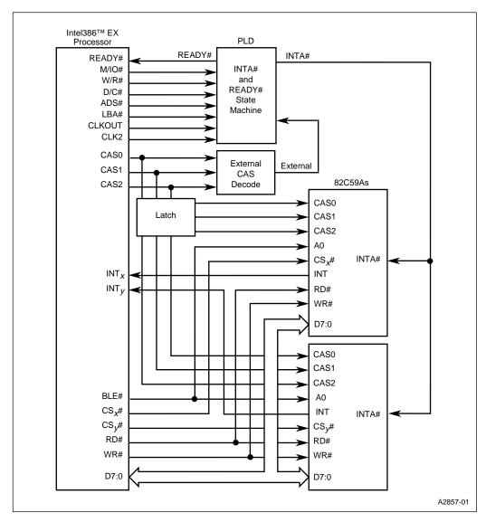
Figure 9-19. Cascading External 82C59A Interrupt Controllers
