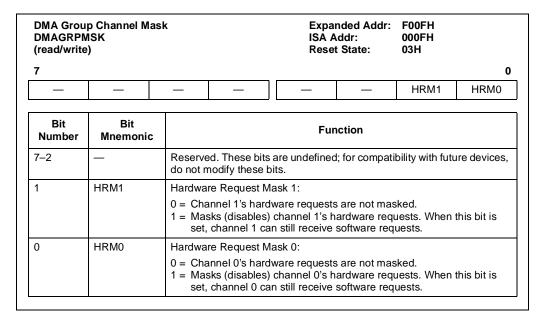
Figure 12-30. DMA Group Channel Mask Register (DMAGRPMSK)
