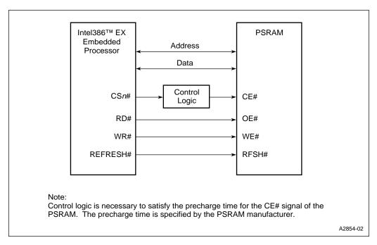
Figure 6-17. Intel386 EX Processor to PSRAM Interface
