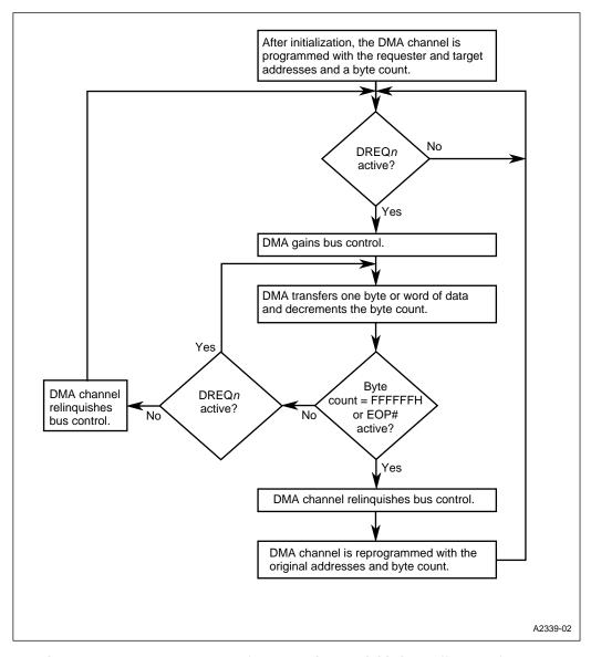
Figure 12-15. Demand Data-transfer Mode with Autoinitialize Buffer-transfer Mode
