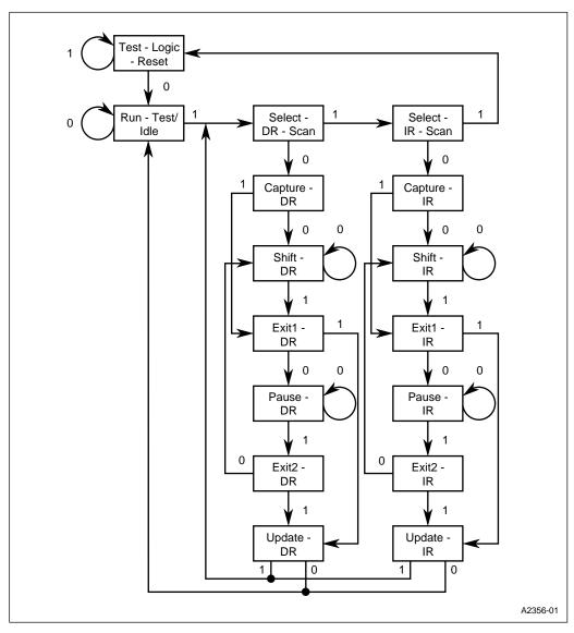
Figure 18-2. TAP Controller (Finite-State Machine)
