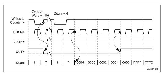
Figure 10-2. Mode 0 - Basic Operation
