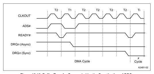
Figure 12-13. Buffer Transfer Suspended by the Deactivation of DRQn
