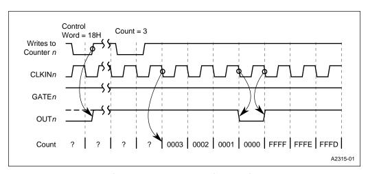
Figure 10-16. Mode 4 – Basic Operation
