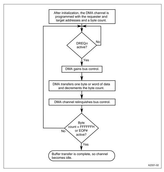
Figure 12-8. Single Data-transfer Mode with Single Buffer-transfer Mode
