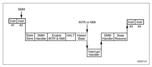
Figure 7-7. HALT During SMM Handler
