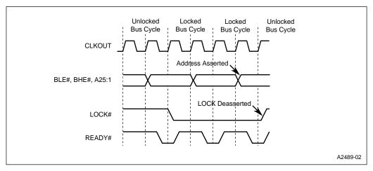
Figure 6-14. LOCK# Signal During Address Pipelining
