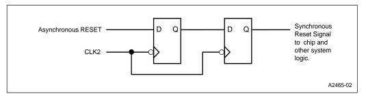
Figure 8-8. Reset Synchronization Circuit
