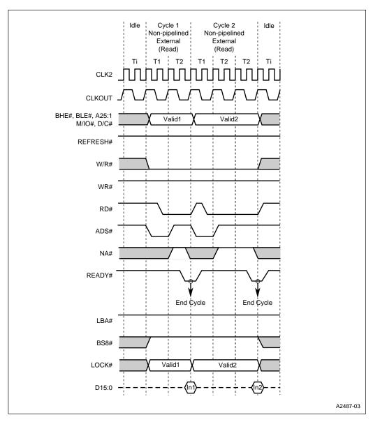
Figure 6-5. Nonpipelined Address Read Cycles
