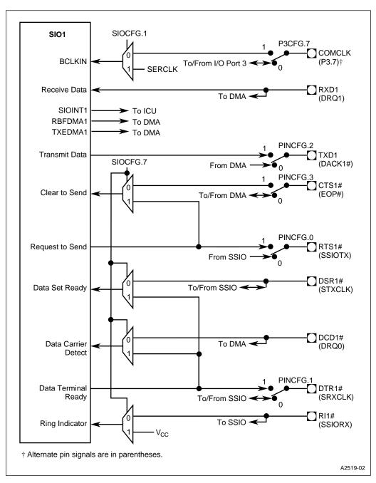
Figure 11-1. Serial I/O Unit 1 Configuration
