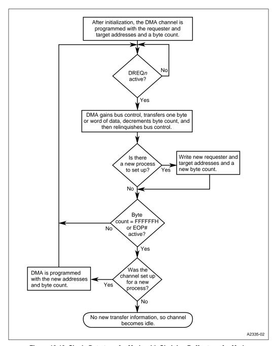
Figure 12-10. Single Data-transfer Mode with Chaining Buffer-transfer Mode
