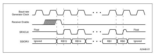
Figure 13-14. Receiver Master Mode, Single Word Transfer
