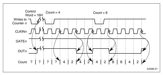
Figure 10-15. Mode 3 – Writing a New Count (Without a Trigger)
