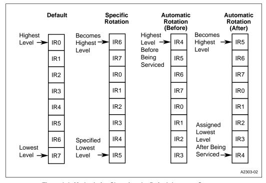
Figure 9-2. Methods for Changing the Default Interrupt Structure
