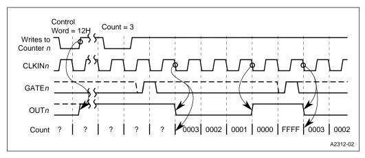
Figure 10-5. Mode 1 - Basic Operation
