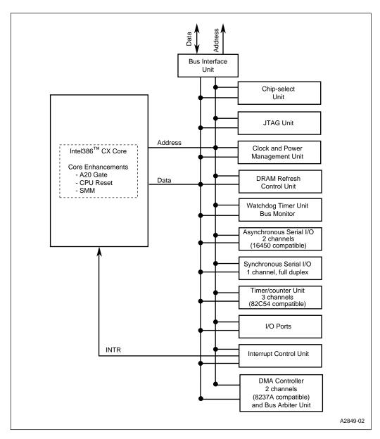
Figure 2-1. Intel386™ EX Embedded Processor Block Diagram
