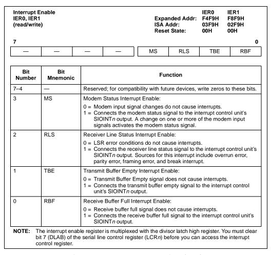
Figure 11-17. Interrupt Enable Register (IERn)
