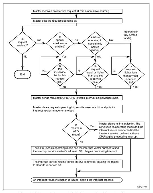
Figure 9-3. Interrupt Process – Master Request from Non-slave Source
