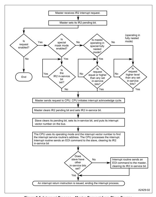
Figure 9-5. Interrupt Process – Master Request from Slave Source
