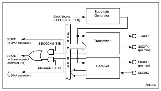
Figure 13-1. Transmitter and Receiver in Master Mode
