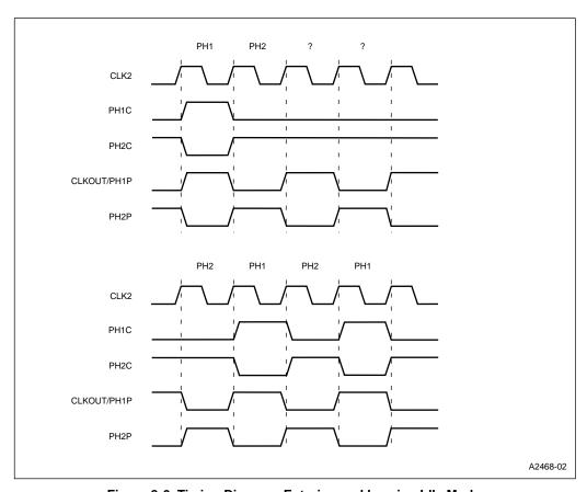
Figure 8-6. Timing Diagram, Entering and Leaving Idle Mode
