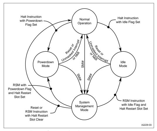
Figure 8-3. SMM Interaction with Idle and Powerdown Modes
