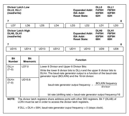
Figure 11-12. Divisor Latch Registers (DLLn and DLHn)
