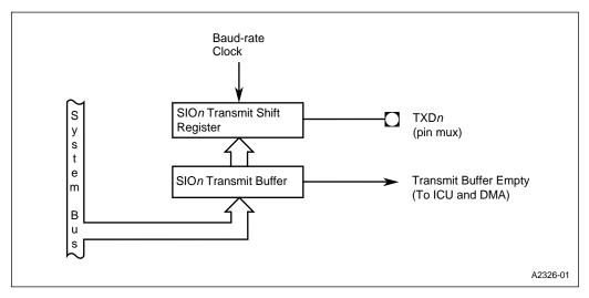
Figure 11-3. SIOn Transmitter
