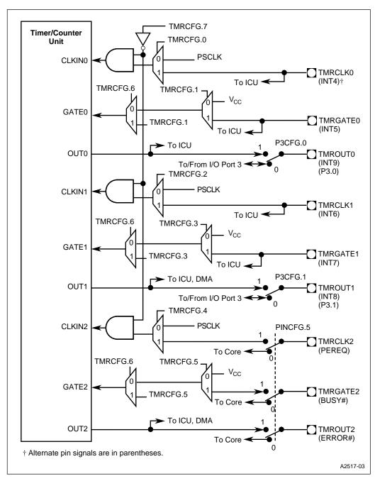
Figure 5-6. Timer/Counter Unit Configuration
