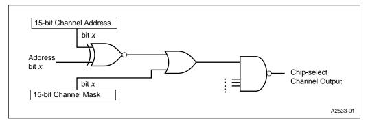
Figure 14-1. Channel Address Comparison Logic
