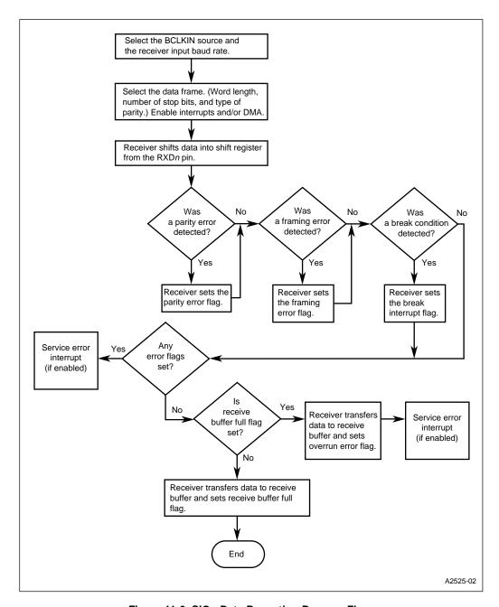
Figure 11-6. SIOn Data Reception Process Flow
