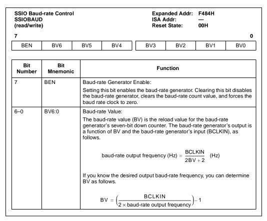
Figure 13-18. SSIO Baud-rate Control Register (SSIOBAUD)
