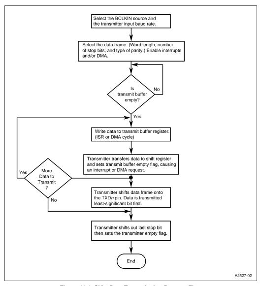
Figure 11-4. SIOn Data Transmission Process Flow
