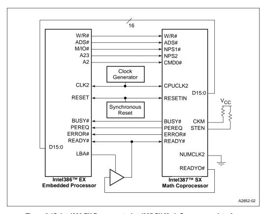
Figure 6-15. Intel386 EX Processor to Intel387 SX Math Coprocessor Interface
