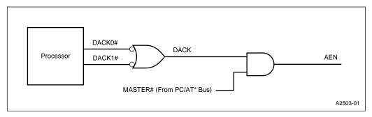
Figure B-2. Derivation of AEN Signal for Intel386™ EX processor-based Systems
