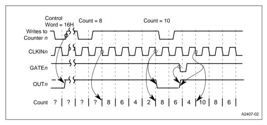
Figure 10-14. Mode 3 – Writing a New Count (With a Trigger)
