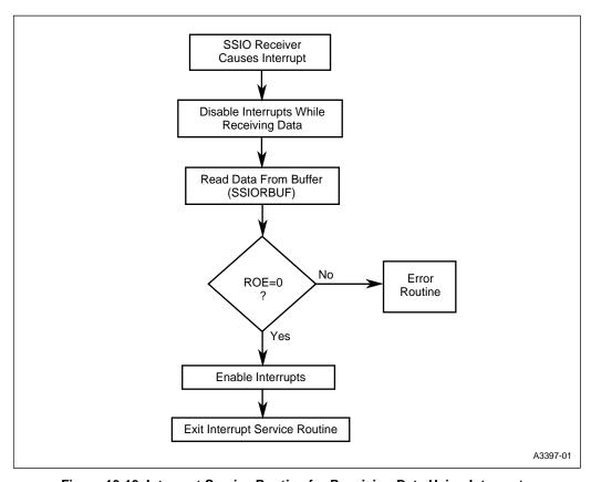
Figure 13-13. Interrupt Service Routine for Receiving Data Using Interrupts
