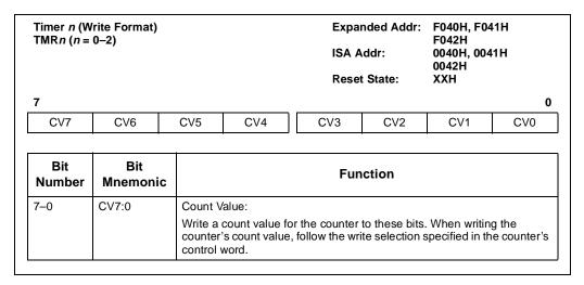
Figure 10-26. Timer *n* Register (TMR*n* – Write Format)
