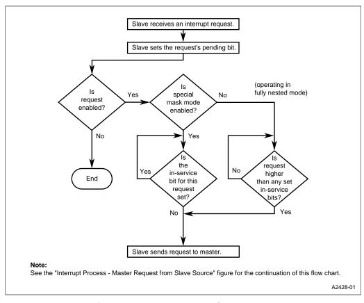
Figure 9-4. Interrupt Process - Slave Request
