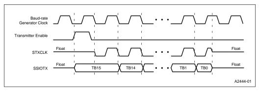
Figure 13-11. Transmitter Master Mode, Single Word Transfer (Enabled when Clock is Low)
