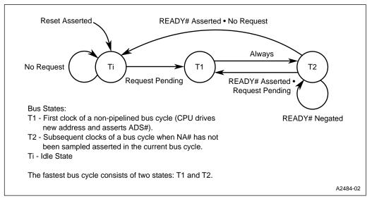
Figure 6-2. Simplified Bus State Diagram (Does Not Include Address Pipelining or Hold states)
