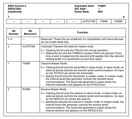
Figure 13-21. SSIO Control 2 Register (SSIOCON2)
