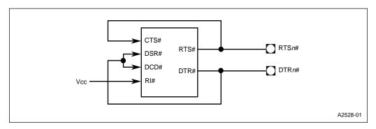
Figure 11-20. Modem Control Signals – Internal Connections
