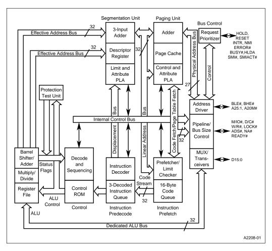
Figure 1. Intel386™ CXSA Microprocessor Block Diagram
