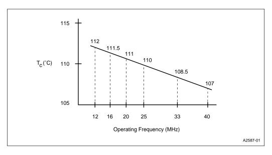
Figure 4. Case Temperature vs. Frequency at  $T_{_{\rm J}}$  = 115° C
