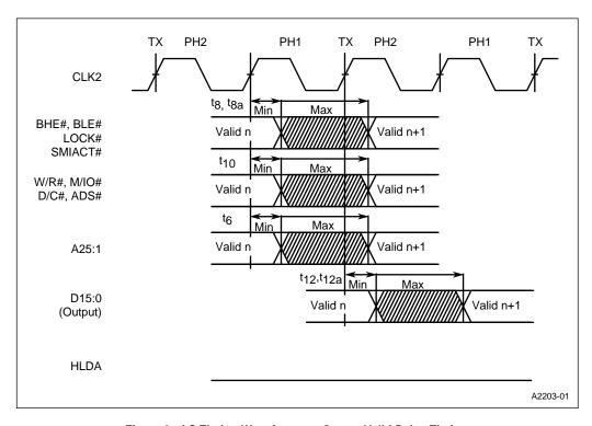
Figure 9. AC Timing Waveforms — Output Valid Delay Timing
