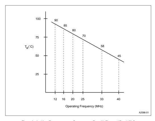
Figure 3. Ambient Temperature vs. Frequency at Zero Air Flow and  $T_{\rm J}$  = 115° C
