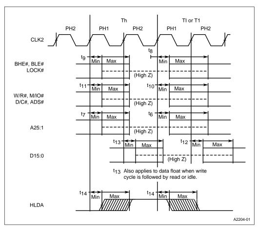
Figure 10. AC Timing Waveforms — Output Float Delay and HLDA Valid Delay Timing
