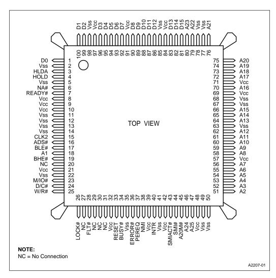
Figure 2. Intel386™ CXSA Microprocessor Pin Assignment (PQFP)
