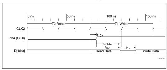
Figure 1. Interfacing the Intel386™ EX Embedded Processor with Intel Flash
