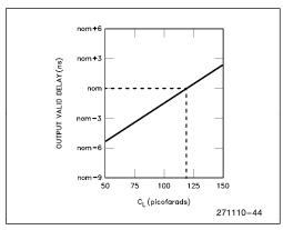
Figure 7.8. Typical Output Valid Delay versus Load Capacitance at Maximum Operating Temperature ( $C_L = 120 \text{ pF}$ )
