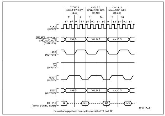
Figure 5.4. Fastest Read Cycles with Non-pipelined Address Timing
