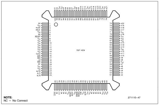
Figure 1.2. i386™ SX Microprocessor Pin Out Top View
