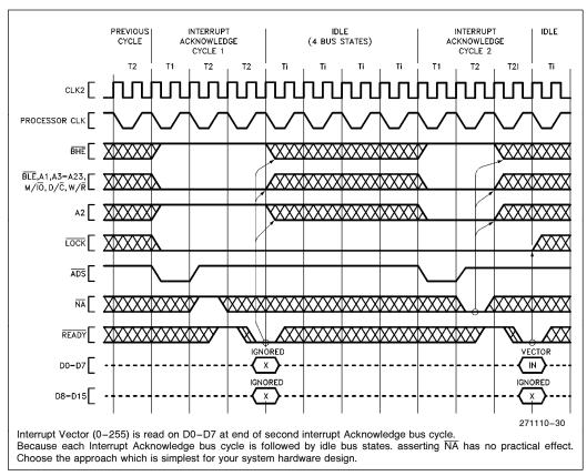
Figure 5.13. Interrupt Acknowledge Cycles
