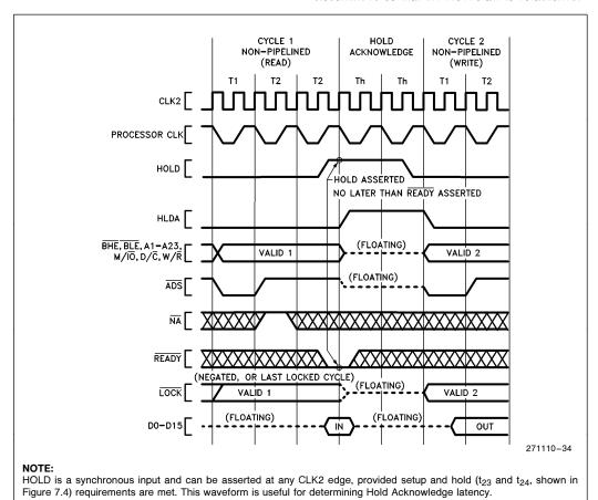
Figure 5.17. Requesting Hold from Active Bus (NA inactive)
