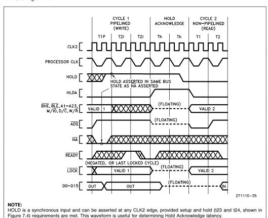
Figure 5.18. Requesting Hold from Idle Bus (NA active)
