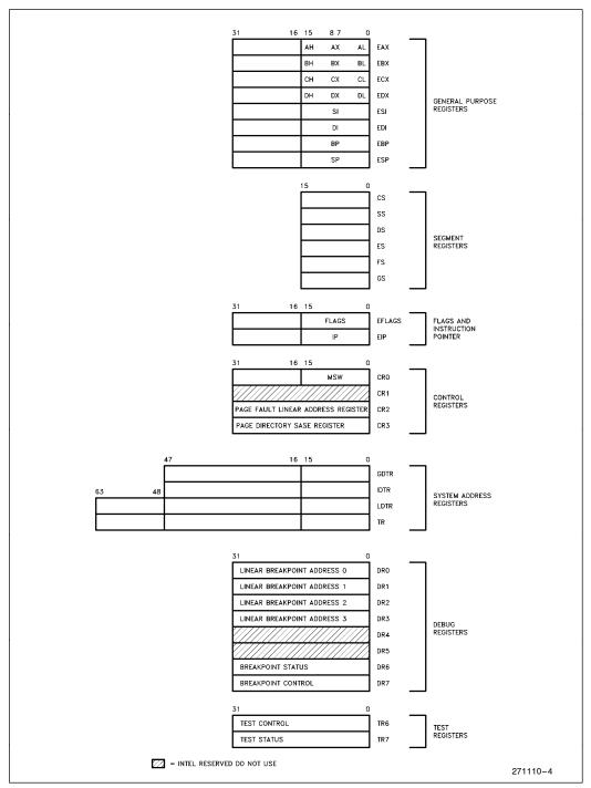
Figure 2.1. i386™ SX Microprocessor Registers
