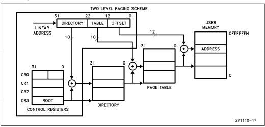
Figure 4.10. Paging Mechanism
