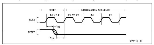
Figure 7.7. AC Timing Waveforms—RESET Setup and Hold Timing and Internal Phase
