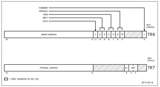
Figure 2.6. Test Registers
