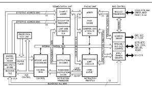
i386™ SX Pipelined 32-Bit Microarchitecture
