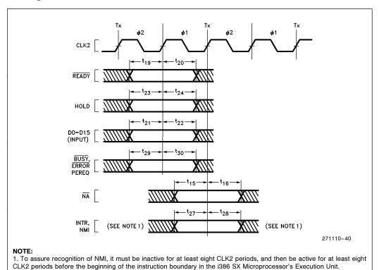
Figure 7.4. AC Timing Waveforms—Input Setup and Hold Timing
