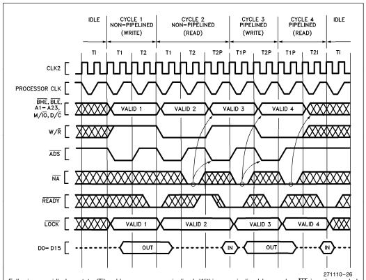
Following any idle bus state (Ti), addresses are non-pipelined. Within non-pipelined bus cycles,  $\overline{\text{NA}}$  is only sampled during wait states. Therefore, to begin address pipelining during a group of non-pipelined bus cycles requires a non-pipelined cycle with at least one wait state (Cycle 2 above).
