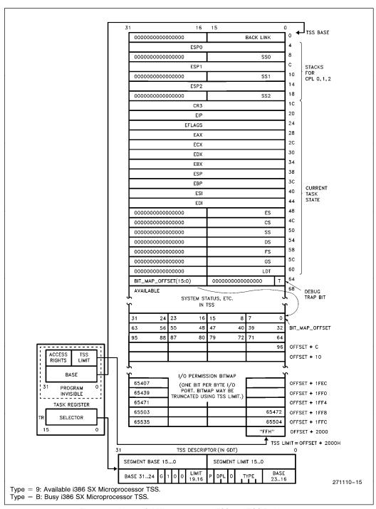
Figure 4.8. i386™ SX Microprocessor TSS and TSS Registers
