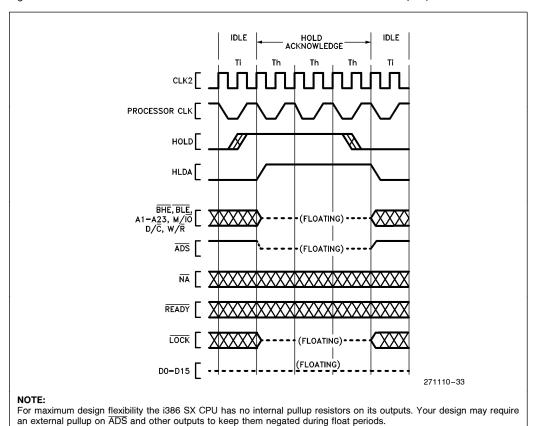
Figure 5.16. Requesting Hold from Idle Bus
