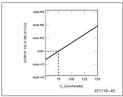
Figure 7.9. Typical Output Valid Delay versus Load Capacitance at Maximum Operating Temperature (C<sub>L</sub> = 75 pF)
