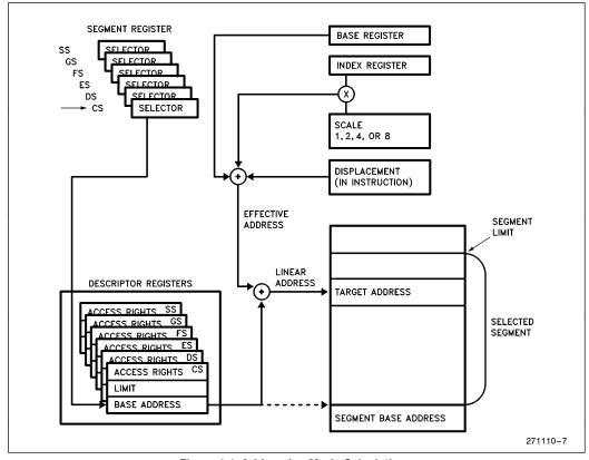
Figure 2.4. Addressing Mode Calculations
