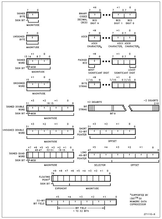
Figure 2.5. i386™ SX Microprocessor Supported Data Types
