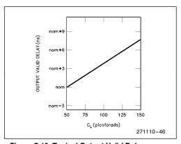
Figure 7.10. Typical Output Valid Delay versus Load Capacitance at Maximum Operating Temperature ( $C_L = 50 \text{ pF}$ )
