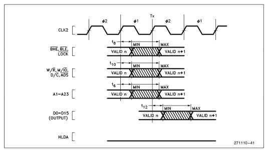
Figure 7.5. AC Timing Waveforms—Output Valid Delay Timing
