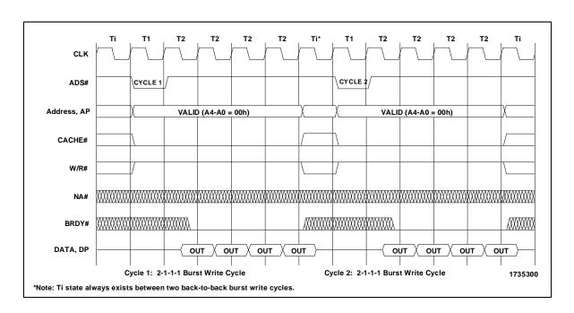
Figure 3-9. Non-Pipelined Burst Write Cycles
