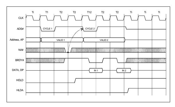
Figure 3-20. Requesting Hold During a Pipelined Bus Cycle
