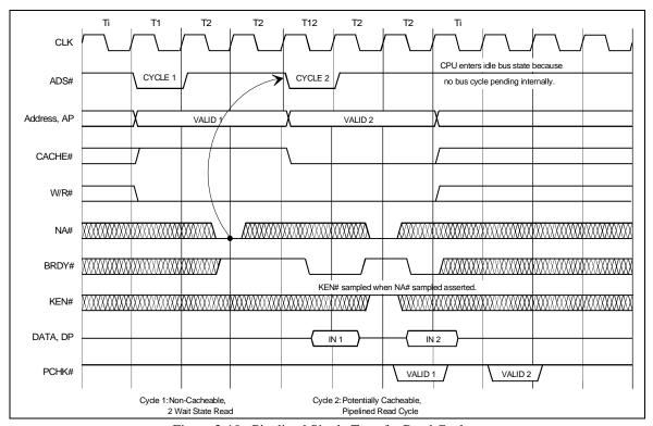
Figure 3-10. Pipelined Single Transfer Read Cycles
