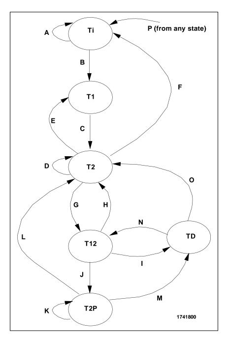
Figure 3-3. IBM 6x86MX CPU Bus State Diagram
