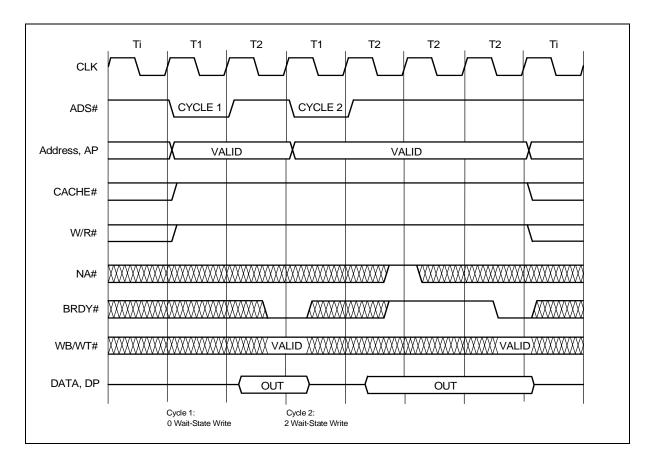
Figure 3-5. Non-Pipelined Single Transfer Write Cycles
