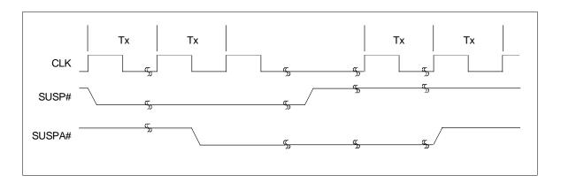
Figure 3-33. Stopping CLK During Suspend Mode
