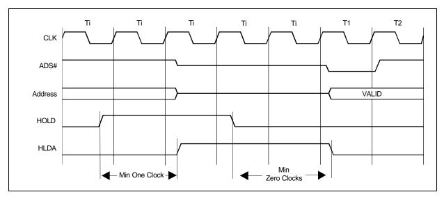
Figure 3-18. Requesting Hold from an Idle Bus
