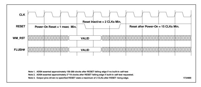
Figure 3-2. RESET Timing
