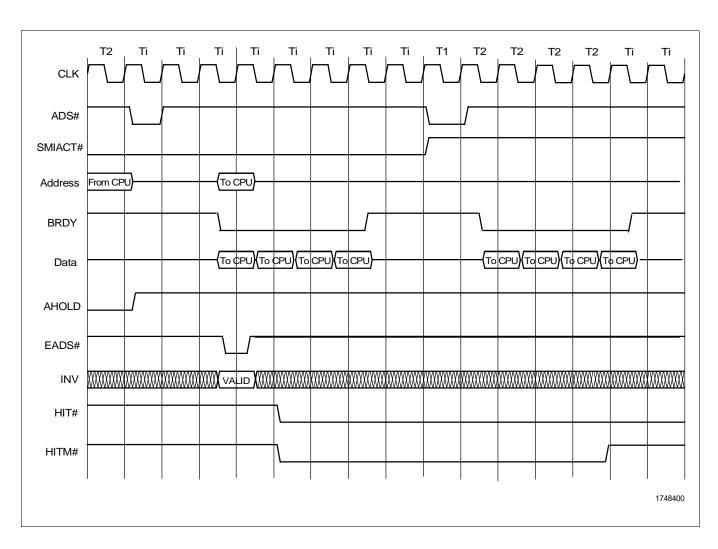
Figure 3-30. AHOLD Inquiry Cycle During a Line Fill from SMM Memory
