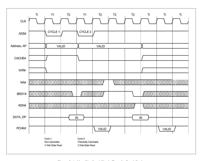
Figure 3-4. Non-Pipelined Single Transfer Read Cycles
