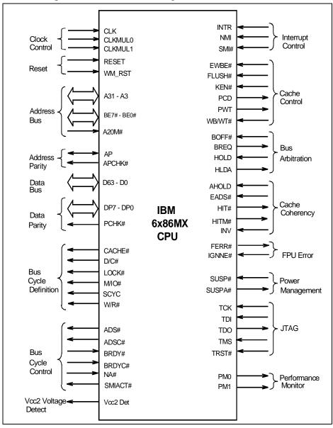
Figure 3-1. IBM 6x86MX CPU Functional Signal Groupings
