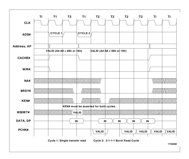
Figure 3-8. "1+4" Burst Read Cycle
