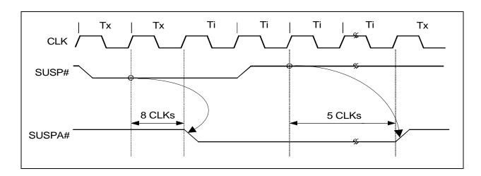
Figure 3-31. SUSP# Initiated Suspend Mode
