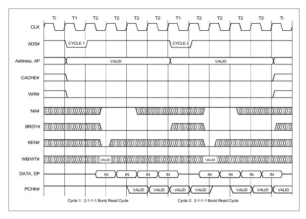
Figure 3-6. Non-Pipelined Burst Read Cycles
