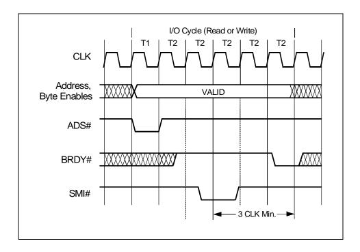
Figure 3-15. SMM I/O Trap Timing
