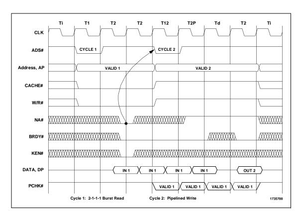
Figure 3-12. Read Cycle Followed by Pipelined Write Cycle
