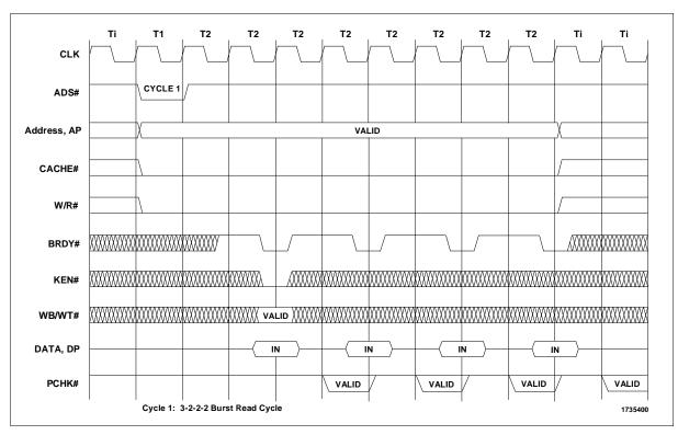
Figure 3-7. Burst Cycle with Wait States
