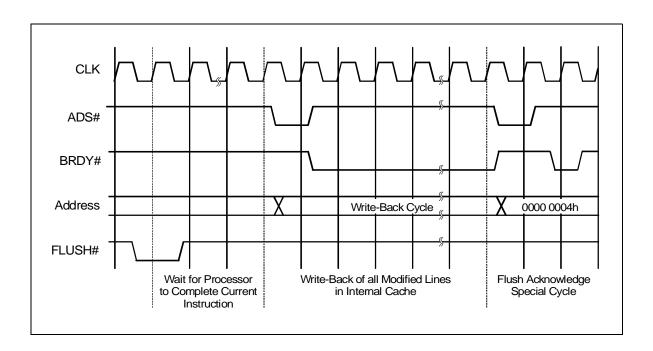
Figure 3-16. Cache Invalidation Using FLUSH#
