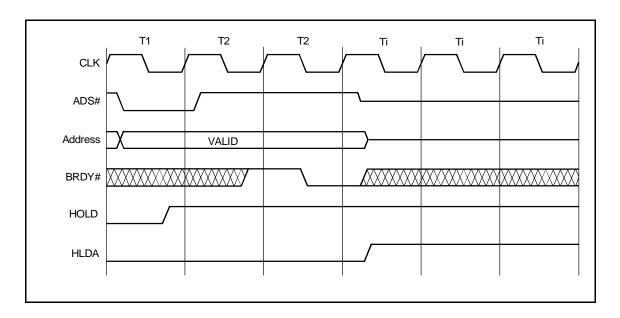
Figure 3-19. Requesting Hold During a Non-Pipelined Bus Cycle
