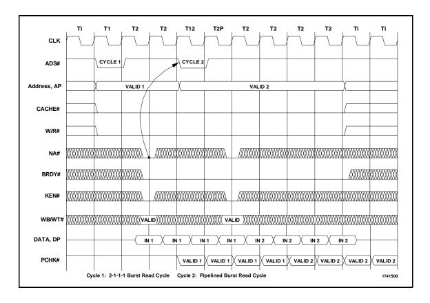
Figure 3-11. Pipelined Burst Read Cycles
