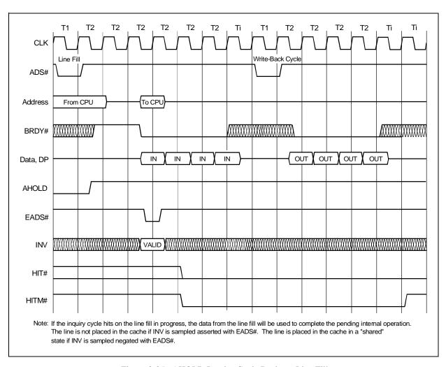
Figure 3-25. AHOLD Inquiry Cycle During a Line Fill
