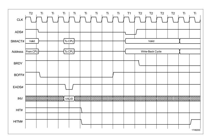
Figure 3-28. BOFF# Inquiry Cycle that Hits on a Modified Data Line
