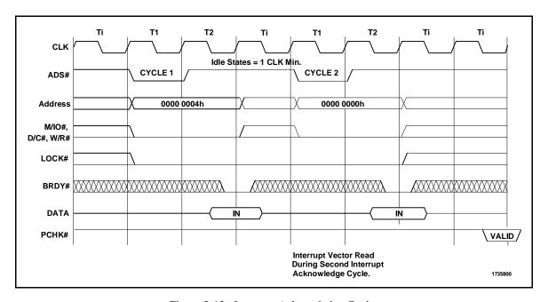
Figure 3-13. Interrupt Acknowledge Cycles
