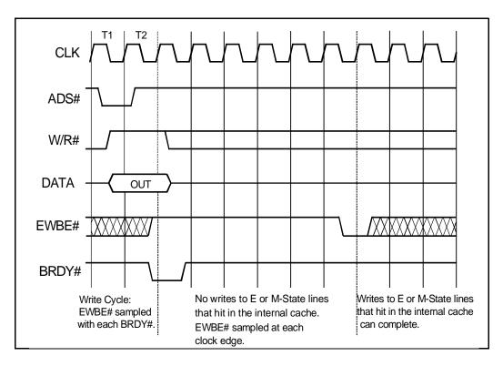
Figure 3-17. External Write Buffer Empty (EWBE#) Timing
