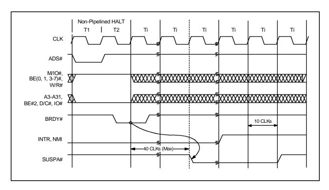
Figure 3-32. HALT Initiated Suspend Mode
