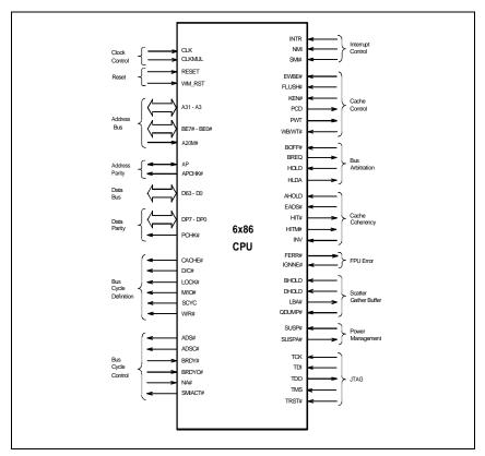
Figure 3-1. IBM 6x86 CPU Functional Signal Groupings
