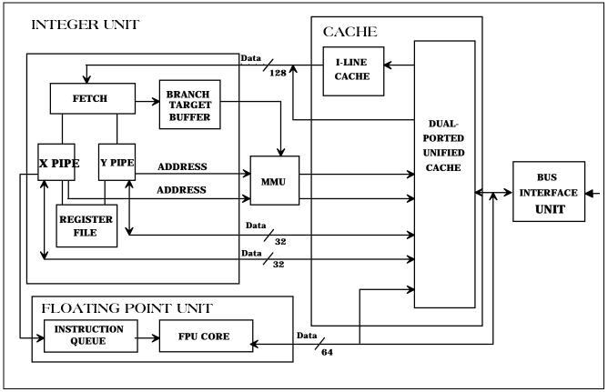
Figure 1. IBM 6x86 and 6x86L Microprocessor Architecture Overview
