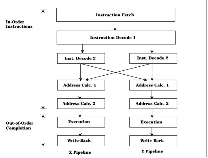
Figure 2. Integer Unit Pipelines
