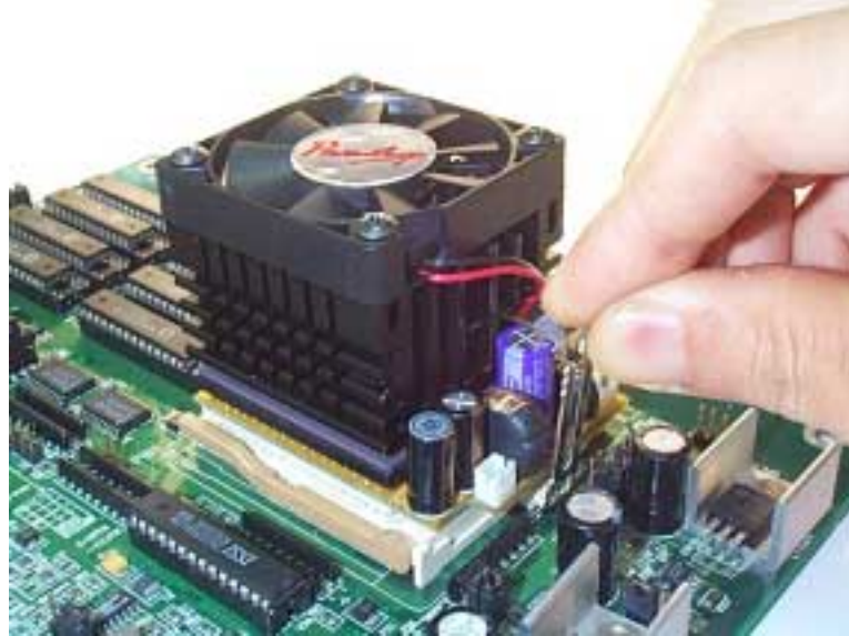
Figure 9. Attaching the retaining bracket (2)
