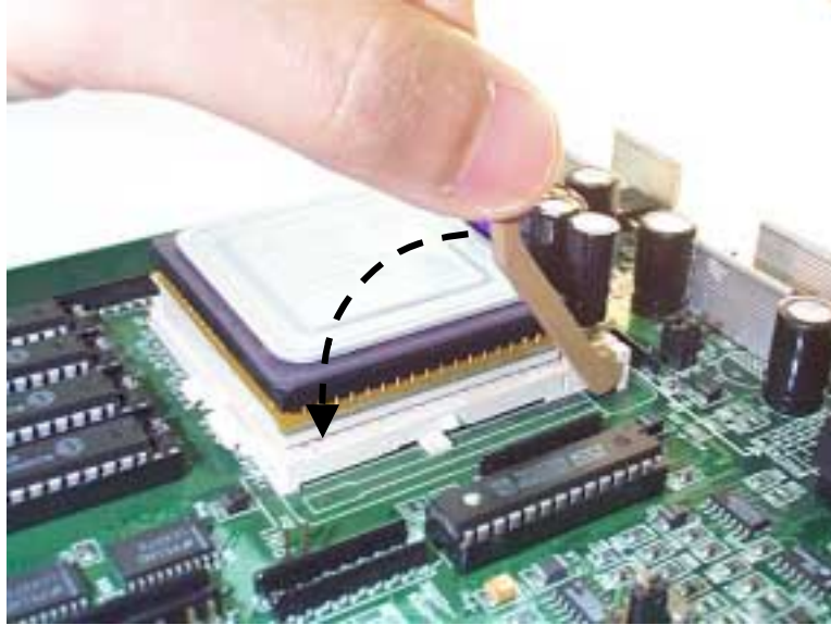
Figure 6. Locking the CPU upgrade adapter into the ZIF socket
