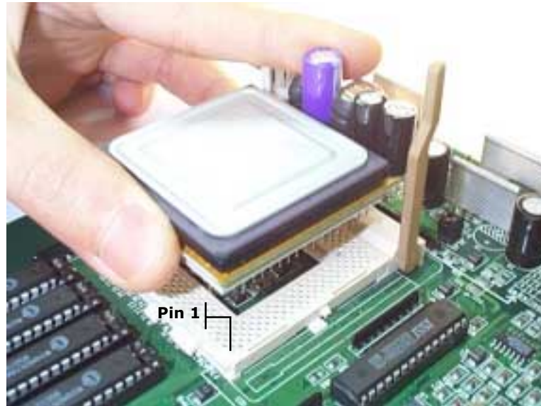
Figure 5. Installing the CPU upgrade adapter into the ZIF socket
