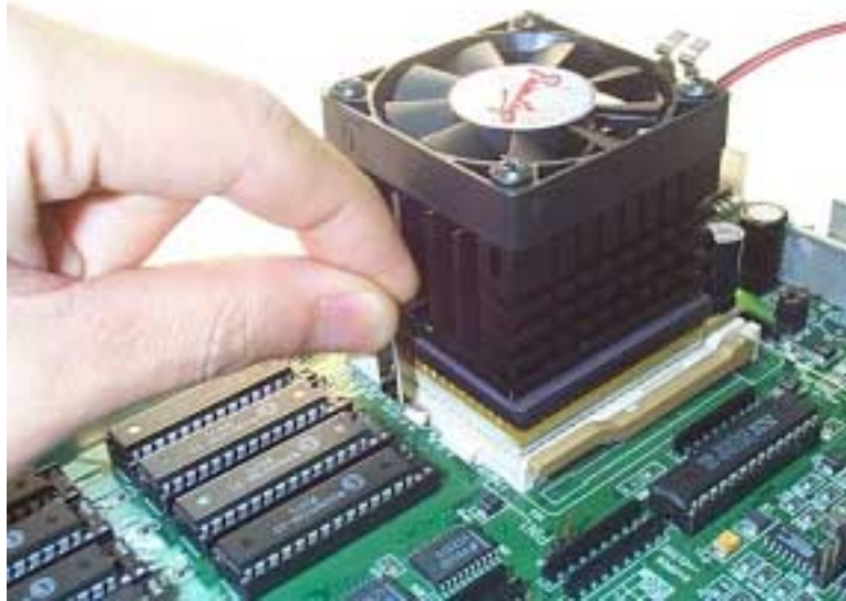
Figure 8. Attaching the retaining bracket (1)
