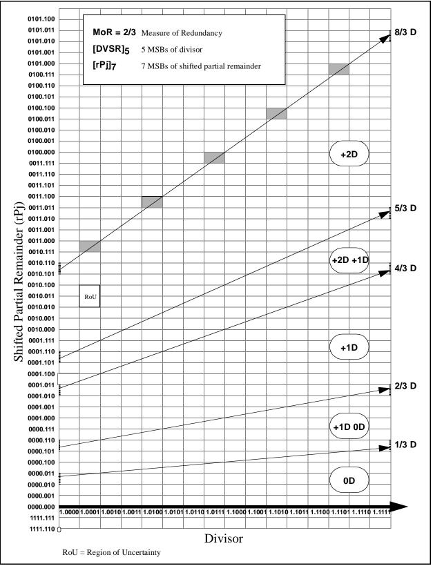
Figure 4-3 Missing Terms in P-D Plot
