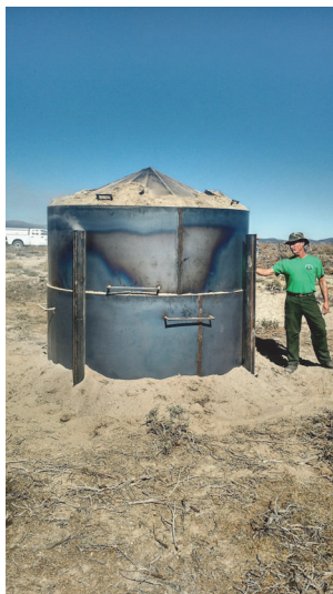
FIGURE 3: Metal kiln being used to process piñon and juniper woody biomass. (Photo credit: E. Roussel.)
