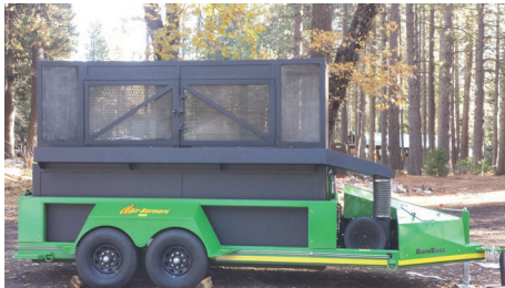
FIGURE 6: Air curtain burner (Photo credit W. Jang, Humboldt State University.)
