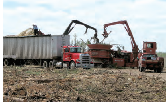
Harvesting fine woody material from jack pine stands is an exception to Guideline 1 because jack pine accumulates less nutrients in comparison to other tree species. In this photo, a jack pine stand is being harvested using a tub grinder. Paul Pingrey, WDNR
