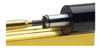
The Forster Neck Reamer will remove excess brass from the inside neck walls of cartridge cases. High-grade tool steel and a staggered-tooth design enable the Forster Neck Reamer to cut brass smoothly without chatter. Forster Neck Reamers are ground .0025"-.003" larger than maximum bullet diameter, therefore neck reaming should be done after the case has been fired with a full load and before the neck or full length sizing operation.
