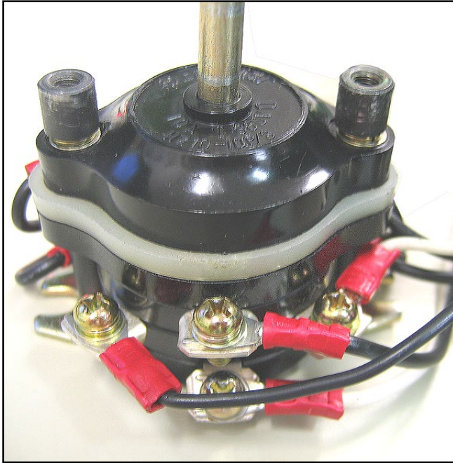
Figure 30. Feed direction switch (Top-side view A).
