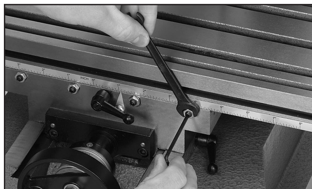
Figure 4. X-axis gib adjustment.
