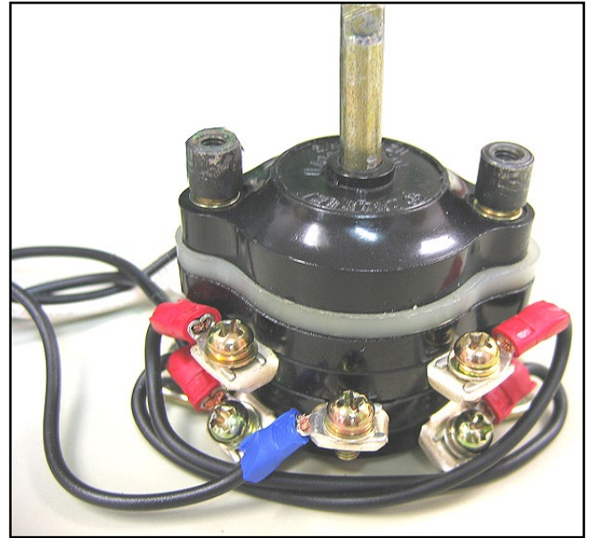
Figure 31. Feed direction switch (Top-side view B).
