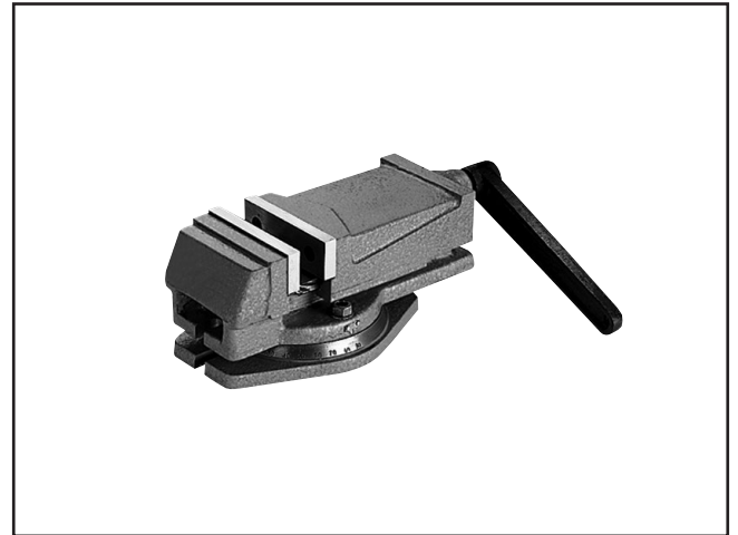
Figure 22. Swivel base milling vise.
