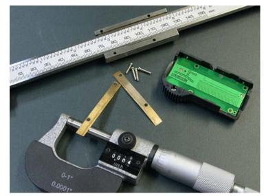
The other assembly will include the encoder circuit board, the battery, the buttons, and the encoder case or shell. This assembly, too, will hang together because the circuit board is held to the encoder case with screws.
