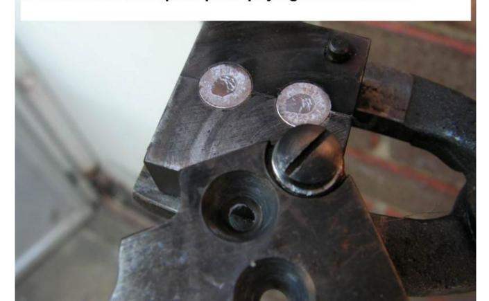
The mold is giving real good fill out from each cavity.
