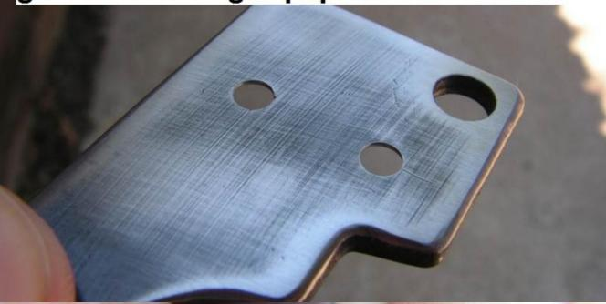
It is not uncommon to find the sprue holes not cut deep enough, they may need to be cut slightly deeper. The sprue holes will quite often times have burrs in them that need cleaning out so the the sprues won't stick. These have been deepened and polished.
