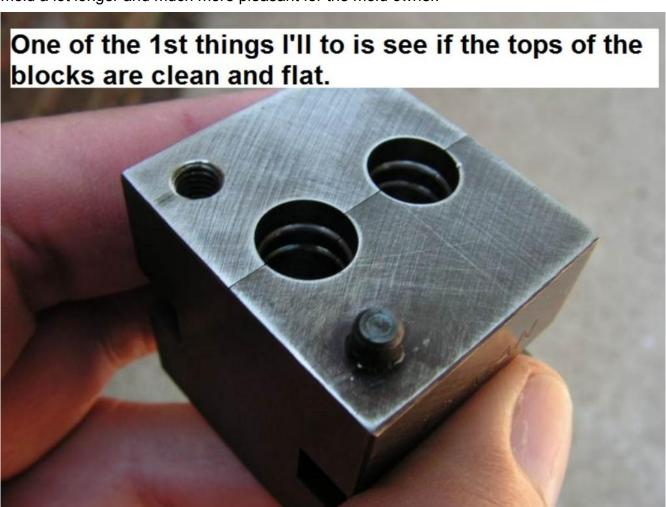
It isn't uncommon to find burrs and raised metal in the sprue bolt hold down threads. I take a counter sink and clean that up.
