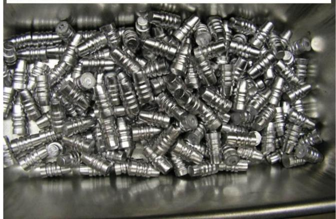
The total amount of time invested in this mold was between 45 minutes and 1 hour. This mold is now a pleasure to use now. No bullets sticking in the cavities, no sprues sticking in the sprue plate holes, great mold fill out and some very nice bullets.
