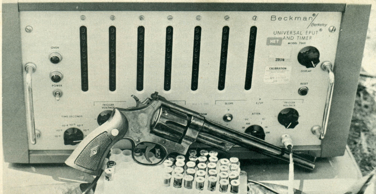
This wildcat handgun was tested, using Beckman electronic instrument to check velocities. A 150-grain bullet was found to travel at 1970 fps.
