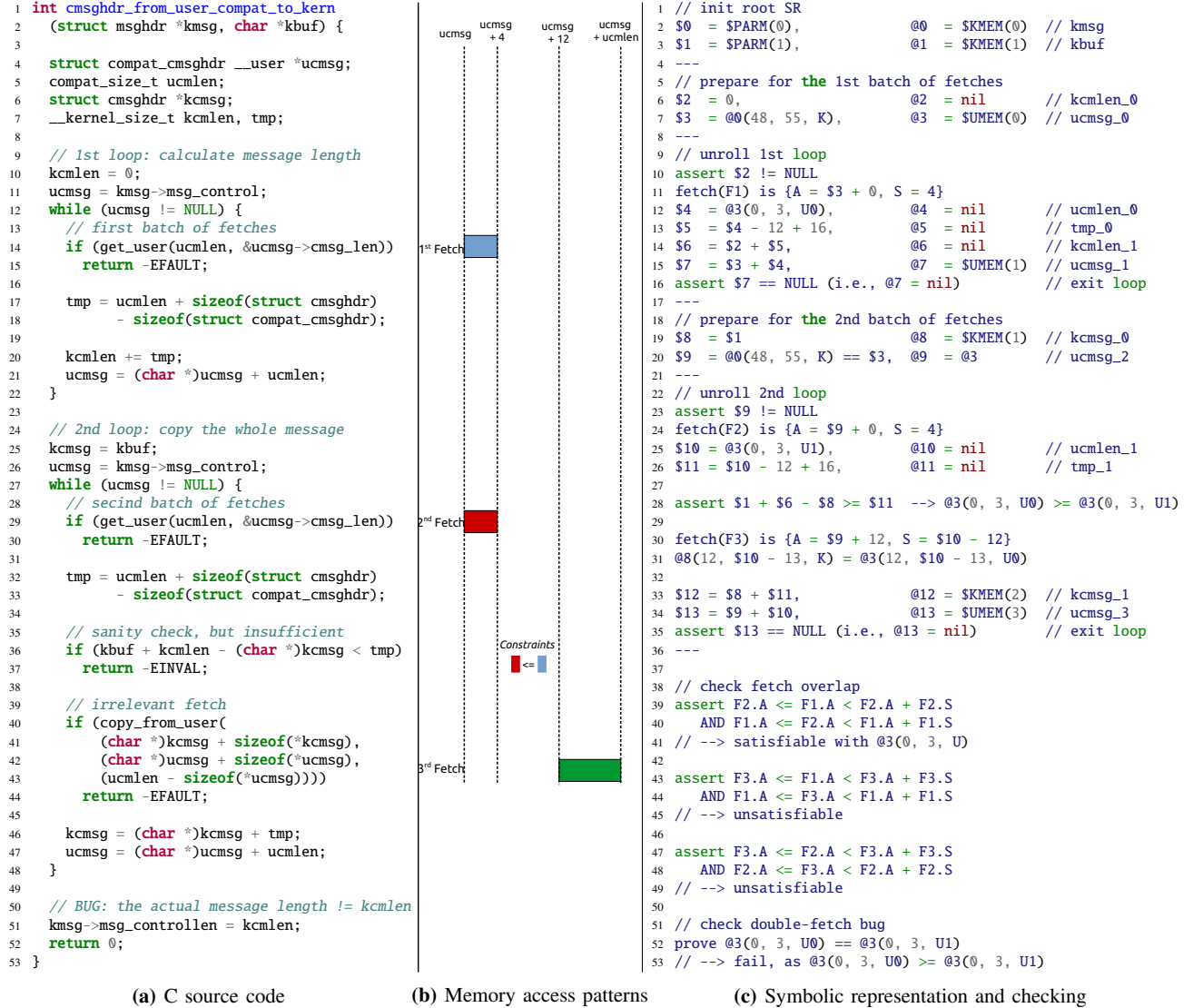
Fig. 7: A double-fetch bug in cmsghdr_from_user_compat_to_kern, with illustration on how it fits the formal definition of double-fetch bugs (7b) and DEADLINE’s symbolic engine can find it (7c).
