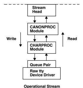
Figure 47. Operational Stream. This diagram shows the raw tty device driver and the queue pair joined. The CHARPROC module is above the queue pair and the CANONPROC module is between the stream head (at the top of the kernel space) and CHARPROC. The modules have the same communication arrows as used in the previous diagram. The upstream queue or read queue is on the right (signified by the upward arrow) while the downstream queue or write queue is on the left (signified by the downward arrow).
