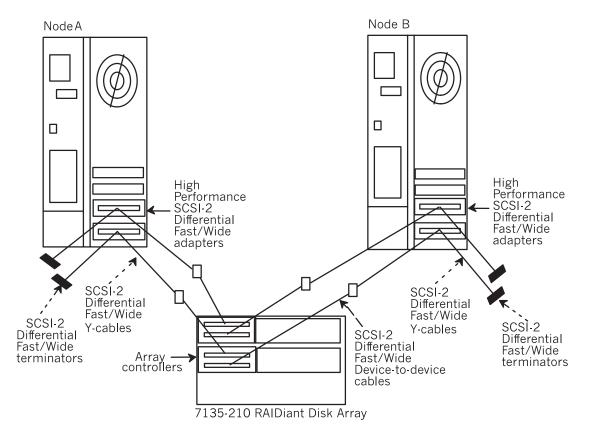
The following figure illustrates an HACMP cluster with an IBM 7135-210 RAIDiant Disk Array connected to two SCSI-2 Differential Fast/Wide buses.
