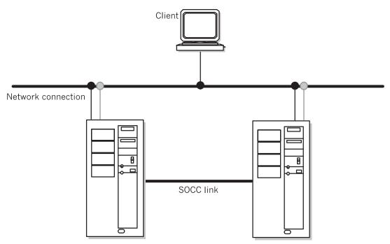
A point-to-point connection directly connects the nodes. This connection is a private network; only neighboring nodes can communicate with each other
