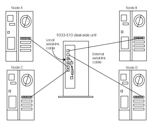
Four-Node Cluster with Shared IBM 9333 Serial Disk Subsystem
