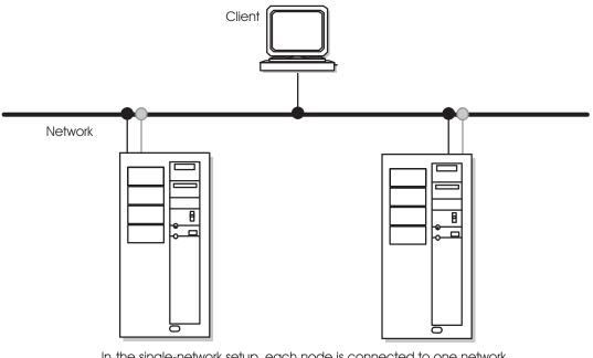
In the single-network setup, each node is connected to one network. Each node has one service adapter and can have none, one, or more standby adapters per public network.
