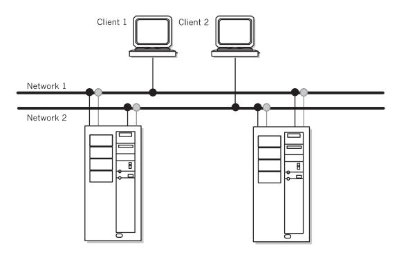
In the dual-network setup, each node is connected to two separate networks. Each node has one service adapter and can have none, one, or more standby adapters per public network.
