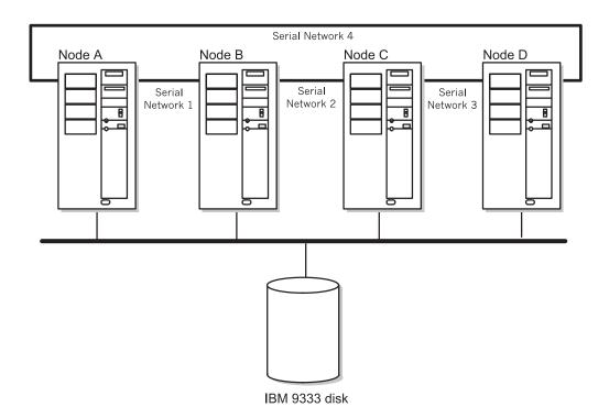
Point-to-Point Serial Networks in a Four-Node Cluster
