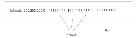
In the preceding figure, the netmask is shown in both dotted decimal and binary format. A binary 1 indicates that a bit is part of the network address. A binary 0 indicates that a bit is part of the host address. In the preceding example, the network portion of the address occupies 24 bits; the host portion occupies 8 bits. It is convenient (but not necessary) to define a subnet on an octet boundary.
