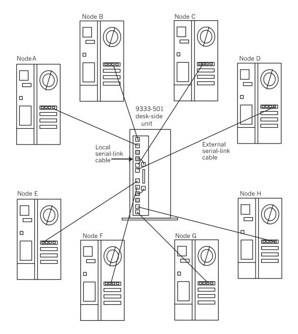
Eight-Node Cluster with Shared IBM 9333 Serial Disk Subsystem
