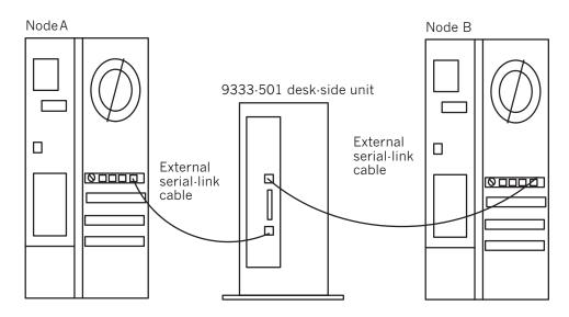
Two-Node Cluster with Shared IBM 9333 Serial Disk Subsystem
