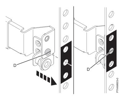
Figure 8. Mounting the rail to the rear of the rack
