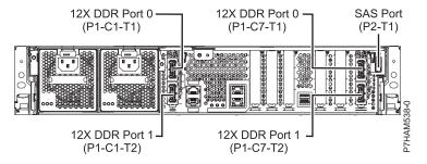
Figure 22. Model 31E/1C or 31E/2C showing all 12X connector locations
