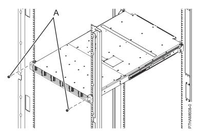
Figure 13. Securing the front of the enclosure to the rack
