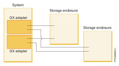
Figure 18. Example of a system that has two GX adapters connected to two storage enclosures for high availability
