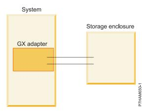
Figure 15. Example of a system that has one GX adapter connected to a single storage enclosure
