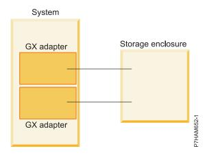
Figure 17. Example of a system that has two GX adapters connected to a single storage enclosure
