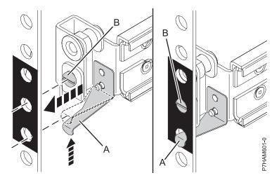
Figure 6. Mounting the rail to the front of the rack
