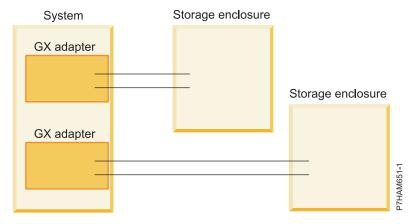
Figure 16. Example of a system that has two GX adapters connected to two storage enclosures
