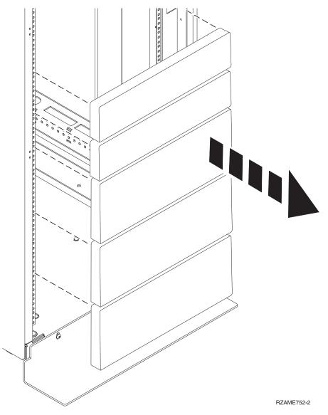
Figure 4. Removing the filler panels
