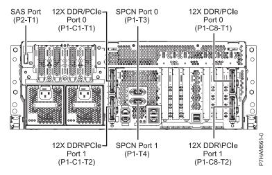
Figure 21. Model 05E/6C connector locations on a rack-mounted model
