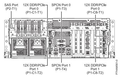
Figure 20. Model 02E/4C connector locations on a rack-mounted model
