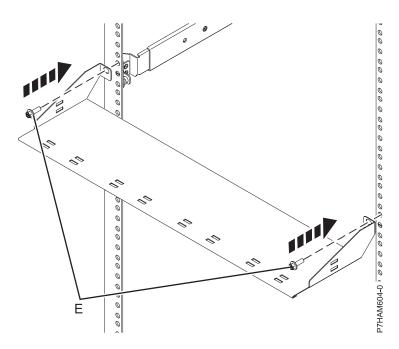
Figure 9. Mounting the cable management bracket
