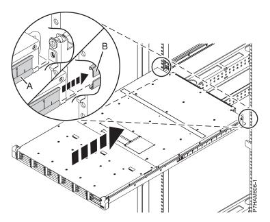
Figure 11. Fitting the enclosure into the rail sheath
