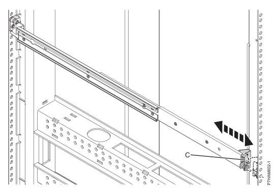
Figure 7. Expanding the rail to the rear of the rack
