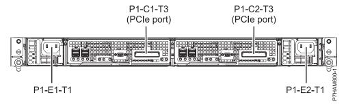
Figure 24. Model 58/88 connector locations
