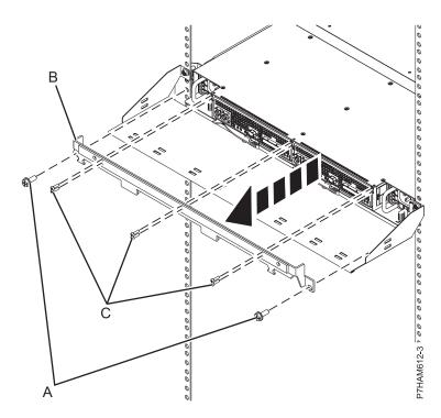
Figure 2. Removing the rear shipping bracket
