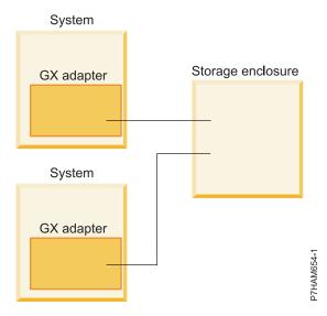
Figure 19. Example of two systems, each with a GX adapter, connected to a single storage enclosure for high availability
