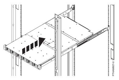
Figure 12. Sliding the disk drive enclosure into the rack
