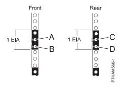
Figure 5. Marking the installation locations
