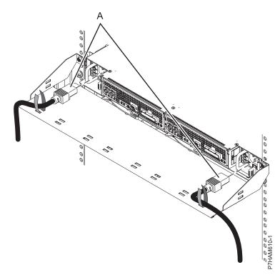
Figure 14. Installing the power cords
