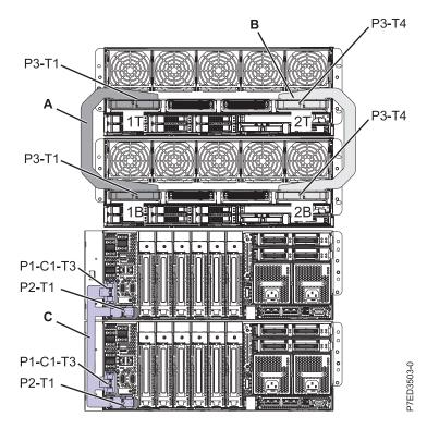
Figure 14. Model 9117-MMB and 9179-MHB 2 drawer flex cabling
