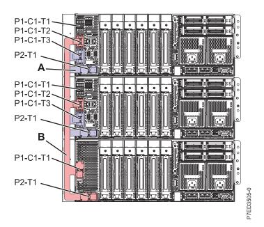
Figure 16. Model 9117-MMB and 9179-MHB 3 drawer flex cabling - rear
