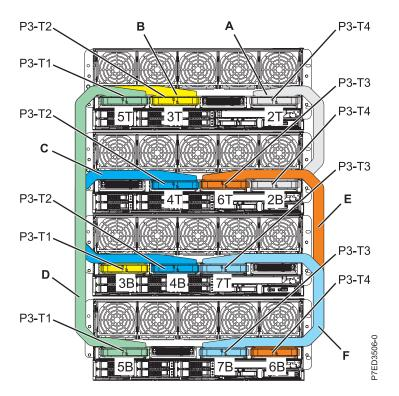
Figure 17. Model 9117-MMB and 9179-MHB 4 drawer flex cabling - front
