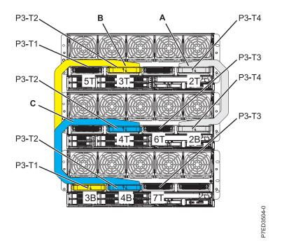
Figure 15. Model 9117-MMB and 9179-MHB 3 drawer flex cabling - front
