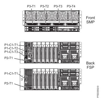
Figure 13. Model 9117-MMB and 9179-MHB multi-drawer flex cabling connector location codes
