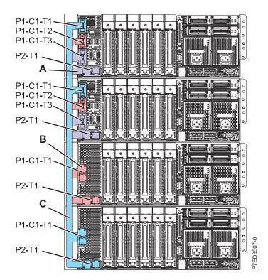
Figure 18. Model 9117-MMB and 9179-MHB 4 drawer flex cabling - rear
