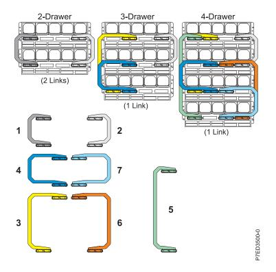
Figure 11. Model 9117-MMB and 9179-MHB multi-drawer SMP flex cabling
