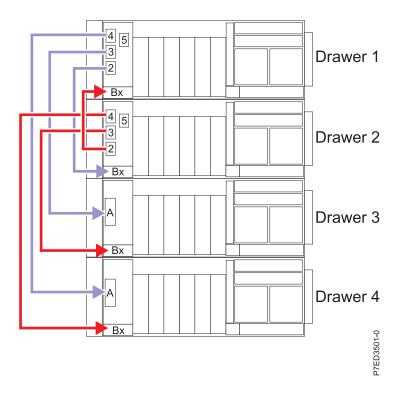
Figure 12. Model 9117-MMB and 9179-MHB multi-drawer FSP flex cabling
