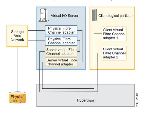
The client can write to the physical storage through client virtual Fibre Channel adapter 1 or 2. If a physical Fibre Channel adapter fails, the client uses the alternative path. This example does not show redundancy in the physical storage, but rather assumes it would be built into the SAN.
