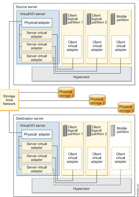
The following figure shows an example of the storage configuration required for partition mobility.
