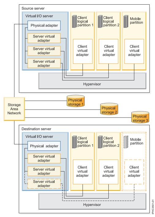
The physical storage that the mobile partition uses, Physical storage 3, is connected to the SAN. At least one physical adapter that is assigned to the source Virtual I/O Server management partition is connected to the SAN, and at least one physical adapter that is assigned to the destination Virtual I/O Server management partition is also connected to the SAN.
